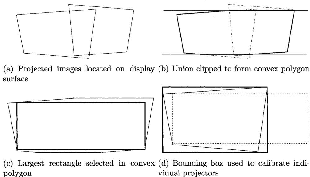
FIGURE 3.1. Geometric calibration of projectors in a large display
