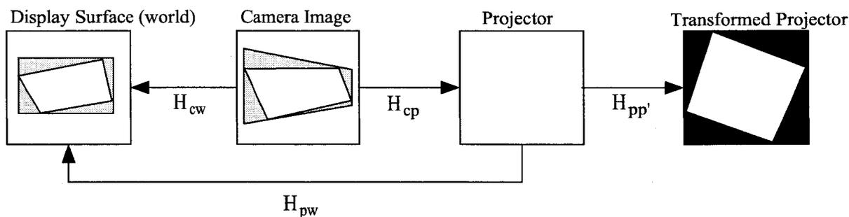
FIGURE 2.1. Different views in the geometric calibration of a single projector
