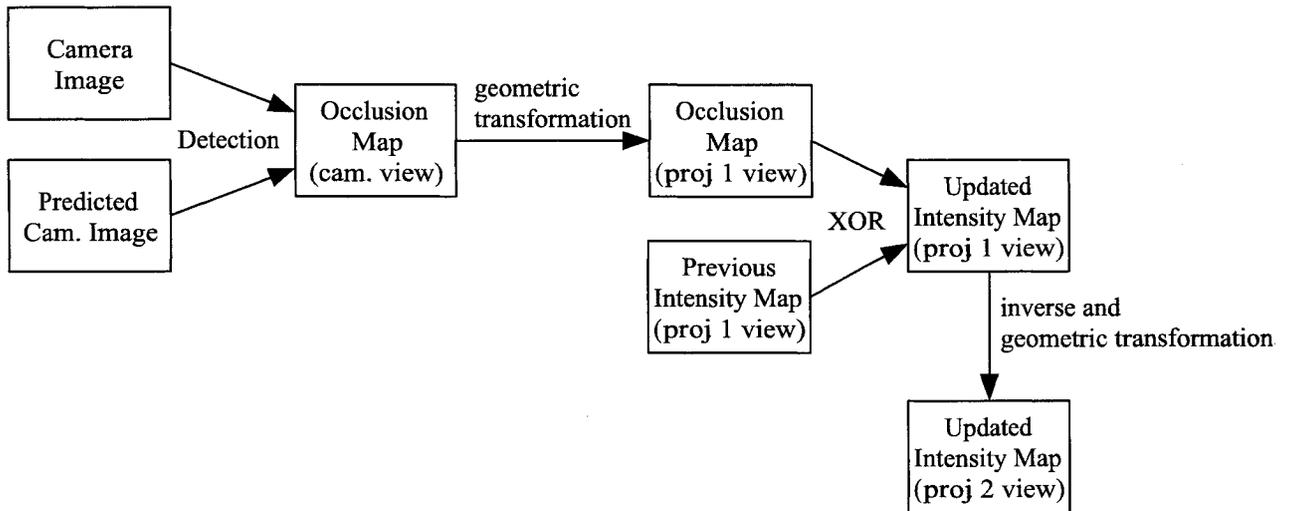
FIGURE 4.1. Process of updating projector intensity maps from detected occlusion
