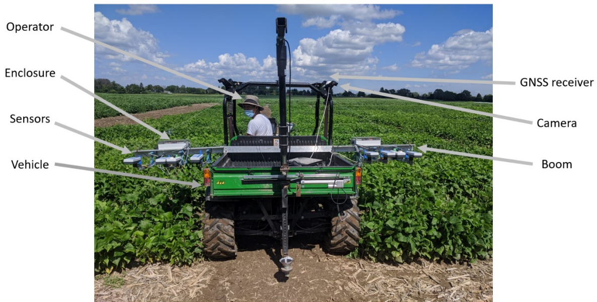
Figure 3-4. Picture of vehicle-mounted HTPP setup
