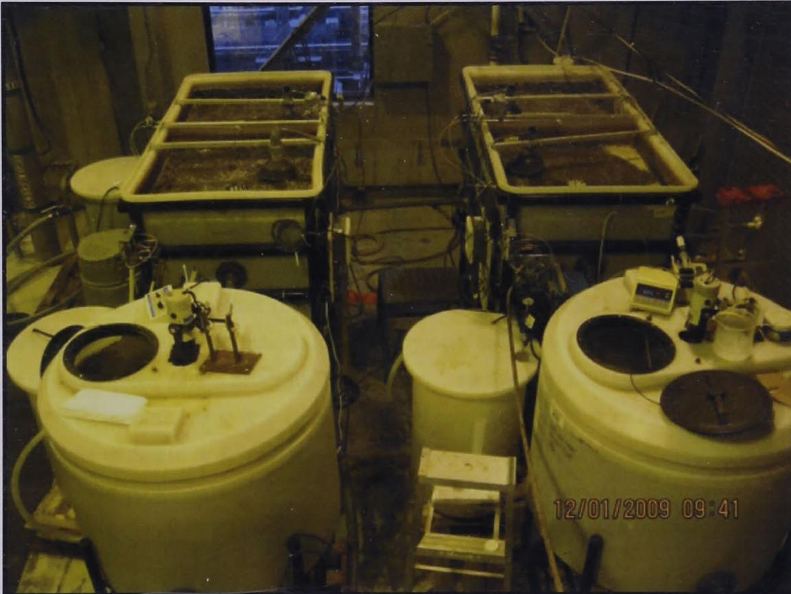
**Figure 8. Wastewater treatment pilot plant, control reactor (right) and ozonated reactor (left)**
