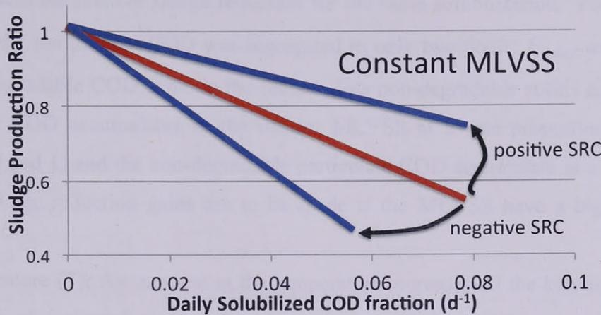
Figure 20. Sludge production ratio slope variation by increase of parameter values
