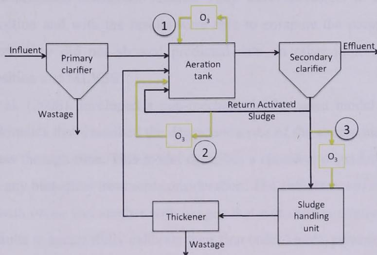
**Figure 6. Three possible ozone reactor configurations (1,2 and 3)**
