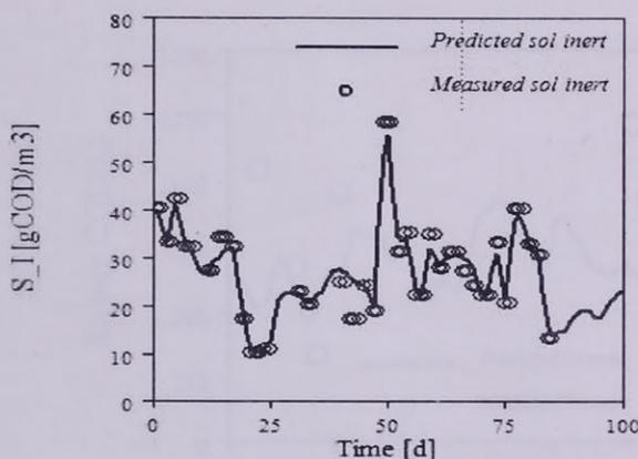
Figure 12. Control reactor effluent soluble inert COD
