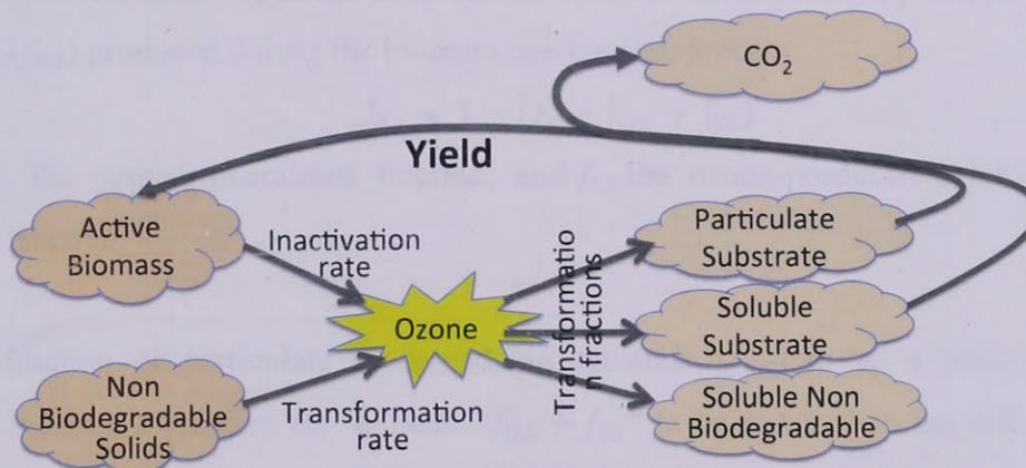
Figure 7. IWA-ASM3 model extension
