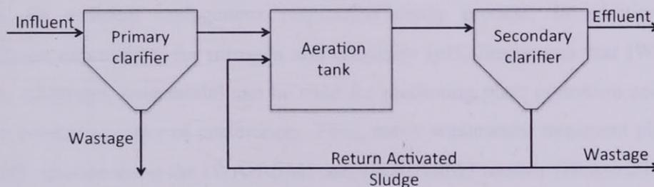
Figure 4. Configuration of a biological wastewater treatment process
