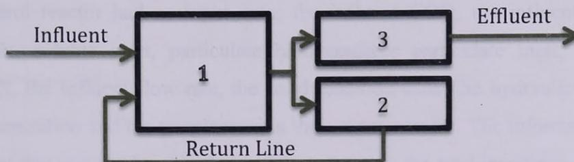
**Figure 9. Simulation program scheme (1-aerated reactor, 2-clarifier bottom section, 3-clarifier top section)**
