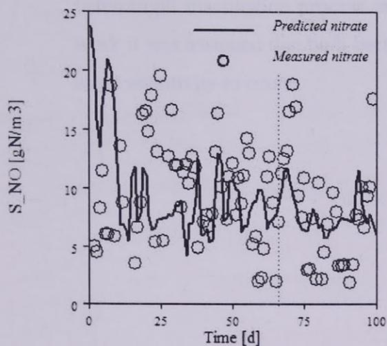
Figure 16. Control reactor effluent nitrate
