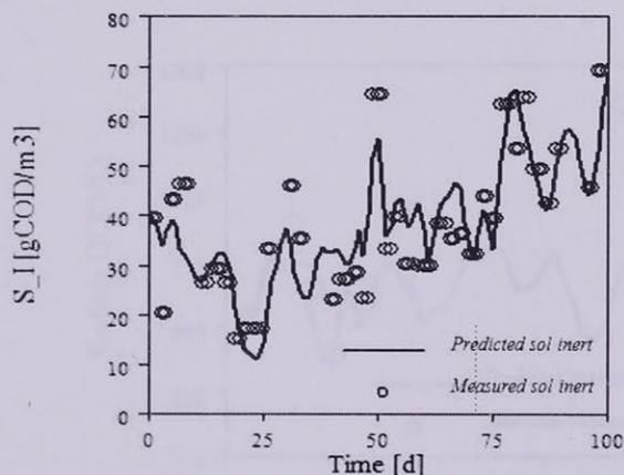
Figure 13. Ozonated reactor effluent soluble inert COD
