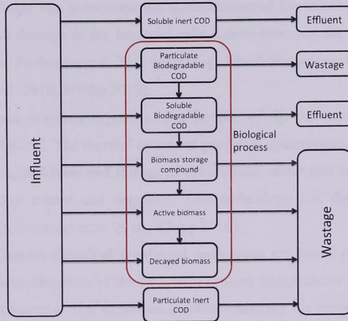
Figure 5. ASM3 schematic
