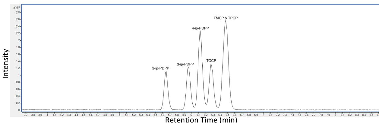
**Figure 3.2** TCP & ip-PDPP isomer separation in pure solvent
