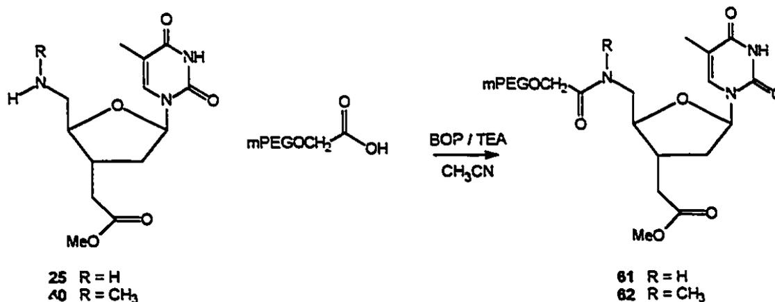
There was, however, a large difference in reaction time. The PEG carboxylic acid was very slow to react. It required three days for the reaction to go to completion, versus 18 hours for dimer **59**, or one hour for non-PEG amide dimers **27** and **47**. Changing the solvent from acetonitrile to DMF made no difference to the reaction rate.
