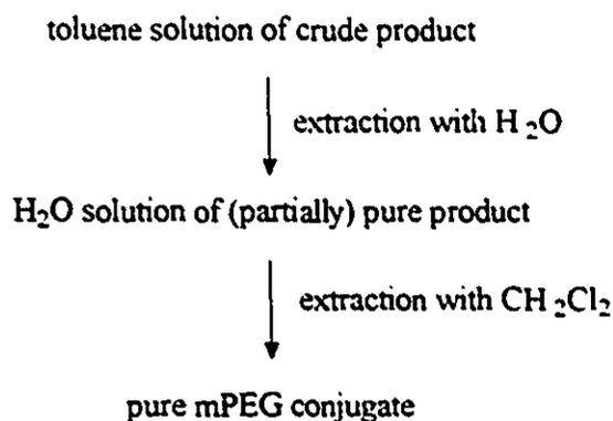
The purification by precipitation from ether was generally found to be convenient and efficient. In cases where the crude reaction mixture contained a lot of salt, purification by extraction was more effective. It was possible to extract PEG adducts preferentially from a toluene solution with water and from a water solution with methylene chloride. The final product could also be recrystallized from ethanol.
