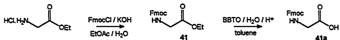
The ethyl ester of glycine.HCl was first reacted with Fmoc chloride under Schotten-Baumann conditions, to yield the corresponding *N*-Fmoc-protected ethyl
