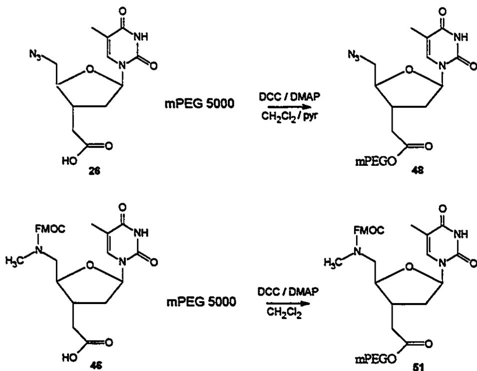
The reaction was monitored by TLC (methylene chloride / methanol, 5 / 1). After two hours no more unreacted PEG could be detected. In order to ensure that the reaction went to completion the reaction mixture was stirred for another hour.
