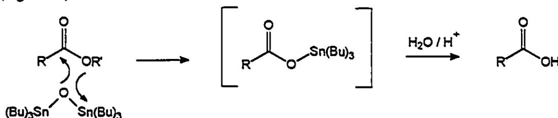
Figure 12. Mechanism for bis(tributyltin) oxide mediated ester cleavage.
