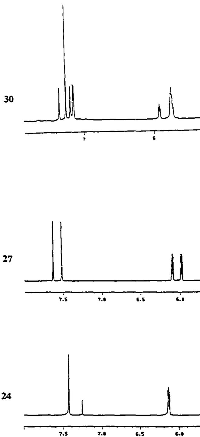
**Figure 13.** Parts of the  $^1\text{H}$  NMR spectra of monomer **24** ( $\text{CDCl}_3$ ), dimer **27** ( $\text{CD}_3\text{OD}$ ), and tetramer **30** ( $\text{CDCl}_3 + \text{CD}_3\text{OD}$ ), showing the signals for  $\text{H1}'$  (around 6 ppm) and  $\text{H6}$  (between 7 and 8 ppm).
