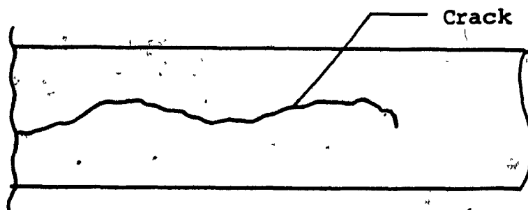
(c) Rapid Crack Propagation (RCP) in Plastic Pipe (Brittle Failure)
