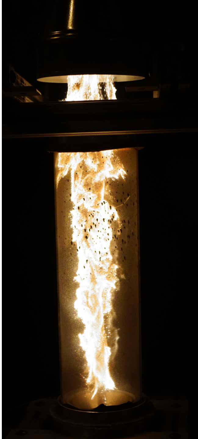
Figure 27: Stabilized Pure Iron Flame Entering Cyclone Ducting
