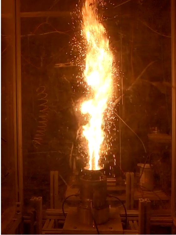
Figure 25: Iron Flame Without Combustion Chamber
