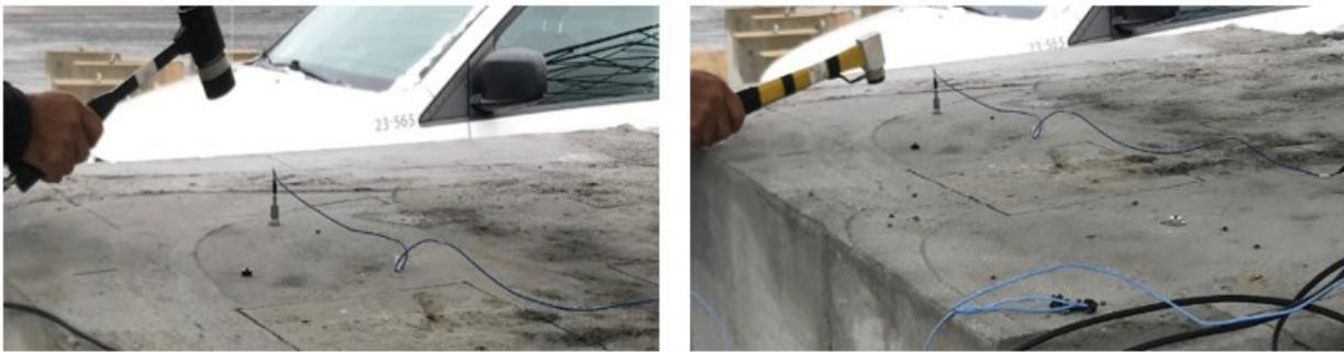
Figure 3-4. Performing impulse-response test with rubber tipped hammer (left) and steel tipped hammer (right).
