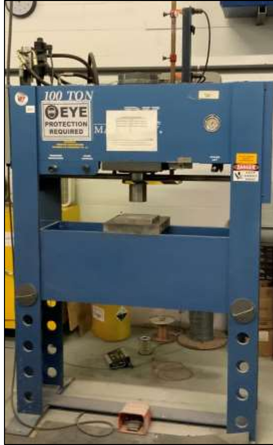
Figure 61: 100 tonne hydraulic press, installed in the MetSim Inc. Stinson Laboratory.
