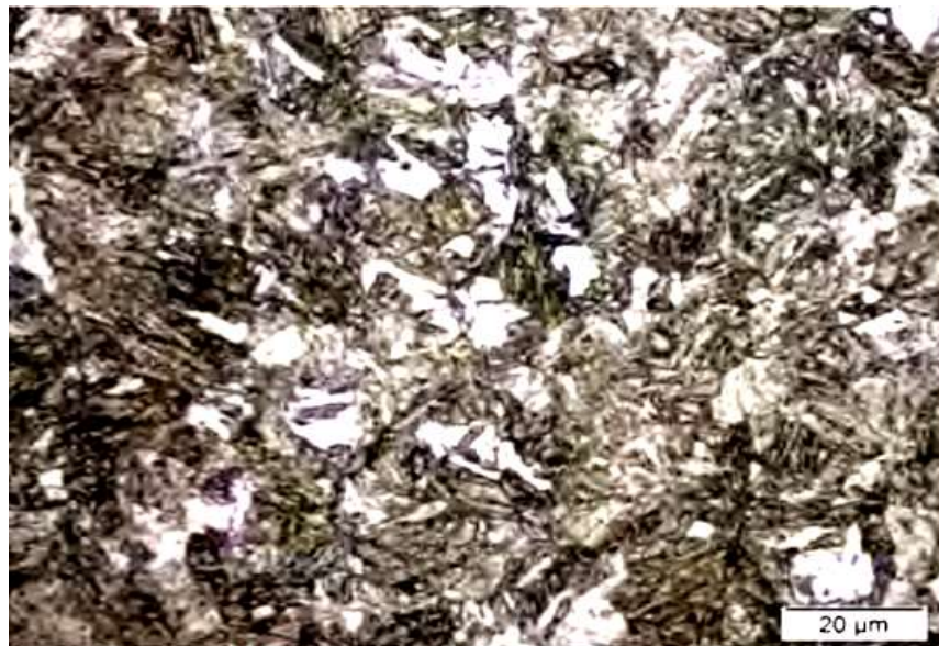
Figure 7: Microstructure of MS Steels, showing a lath martensite structure [64].
