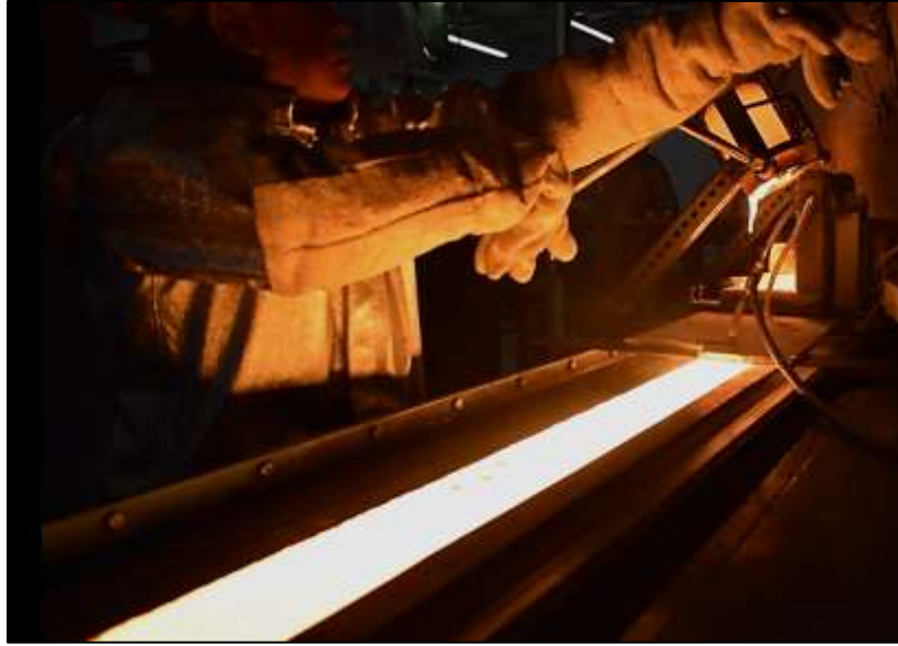
Figure 4. An experiment casting AHSS steel on the pilot-scale HSBC machine.
