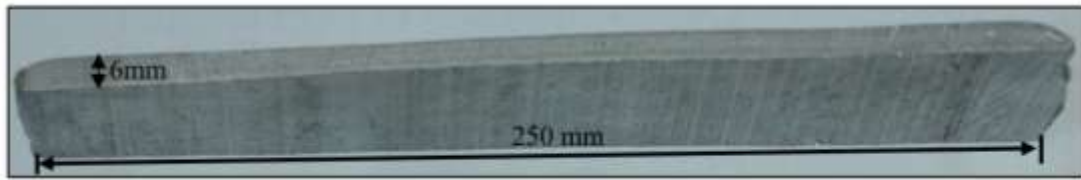
Figure 11: Transverse section of the cast strip.
