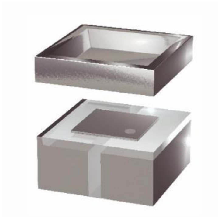
Figure 12 - Exploded View of Murata's Capacitive Pressure Sensor [22]
