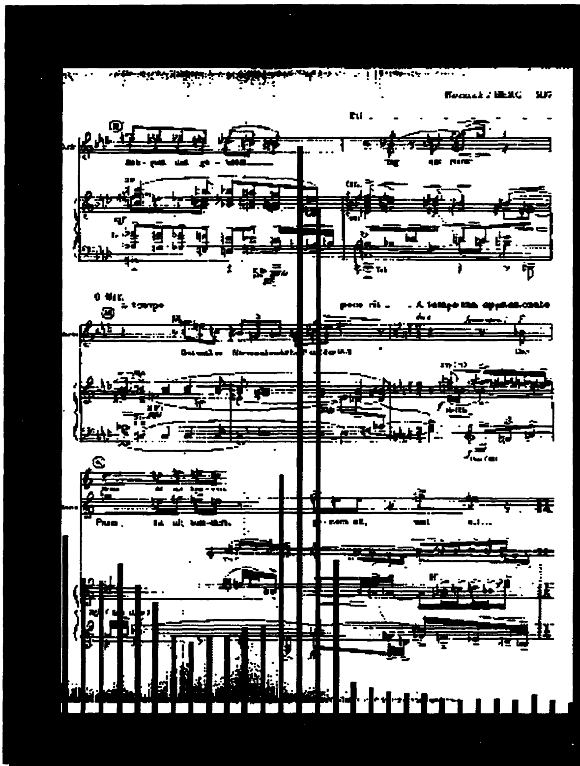
Figure 4.7 Estimating staffspace_height by vertical white runs. The graph shows that the staffspace_height of 14 pixels is most prominent.
