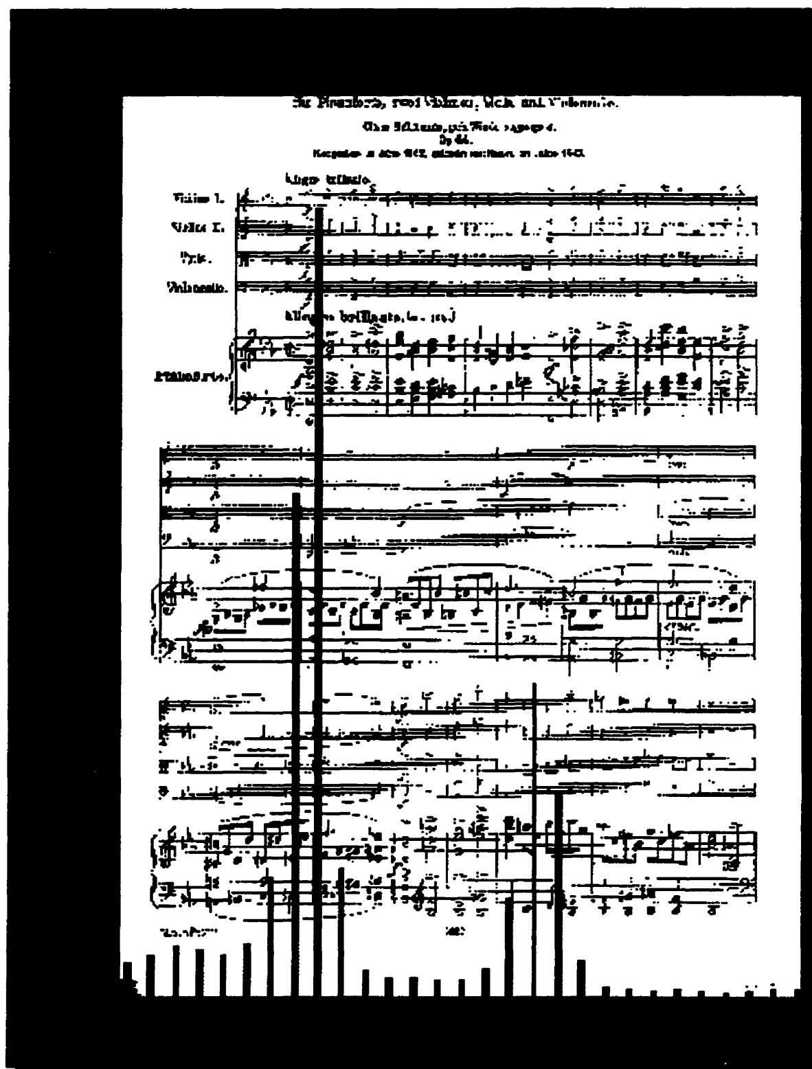
Figure 4.8 Estimating staffspace_height by vertical white runs with multiple-size staves.
