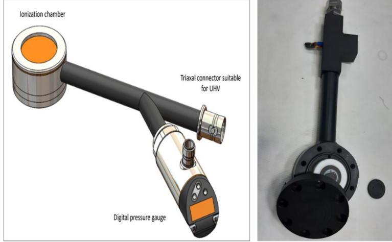
Figure 4.3: Left: A conceptualization of the ALLS chamber design. Right: A prototype ALLS chamber. Reproduced under the Creative Commons CC-BY-NC-ND license from [31].
