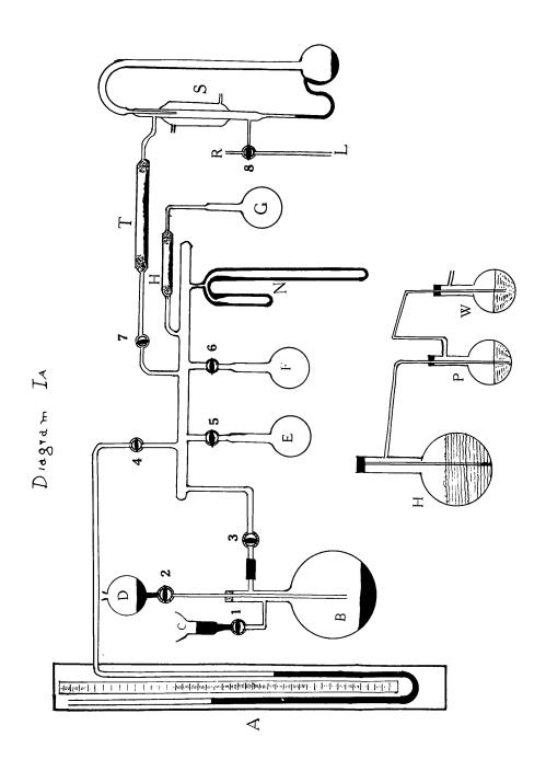
The 200 c.cs. of sulfuric acid which was to be used was also cooled in the same bath and then added in about 25 c.cs. portions and evenly mixed and cooled between additions. When the whole amount of the acid had been added in this way the flask was fitted with a cork stopper, thermometer and delivery tube which dipped beneath the surface of 50 c.cs. of concentrated sulfuric acid (P) and thence to another container with another 50 c.cs. of sulfuric acid (W). (See diagram 1B).
