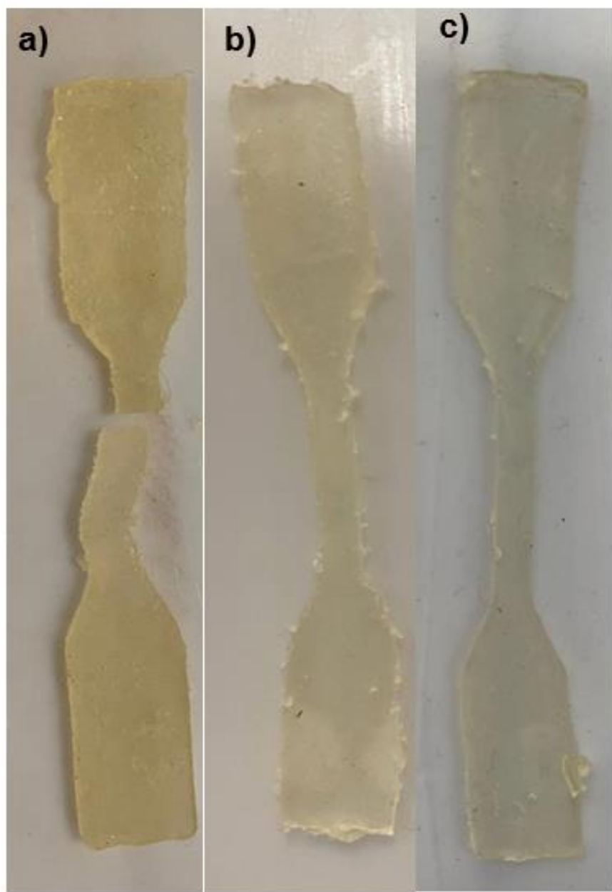
Figure A 14. Tensile bars for the synthesized films, a) EC-70, b) EC-80 and c) EC-90.
