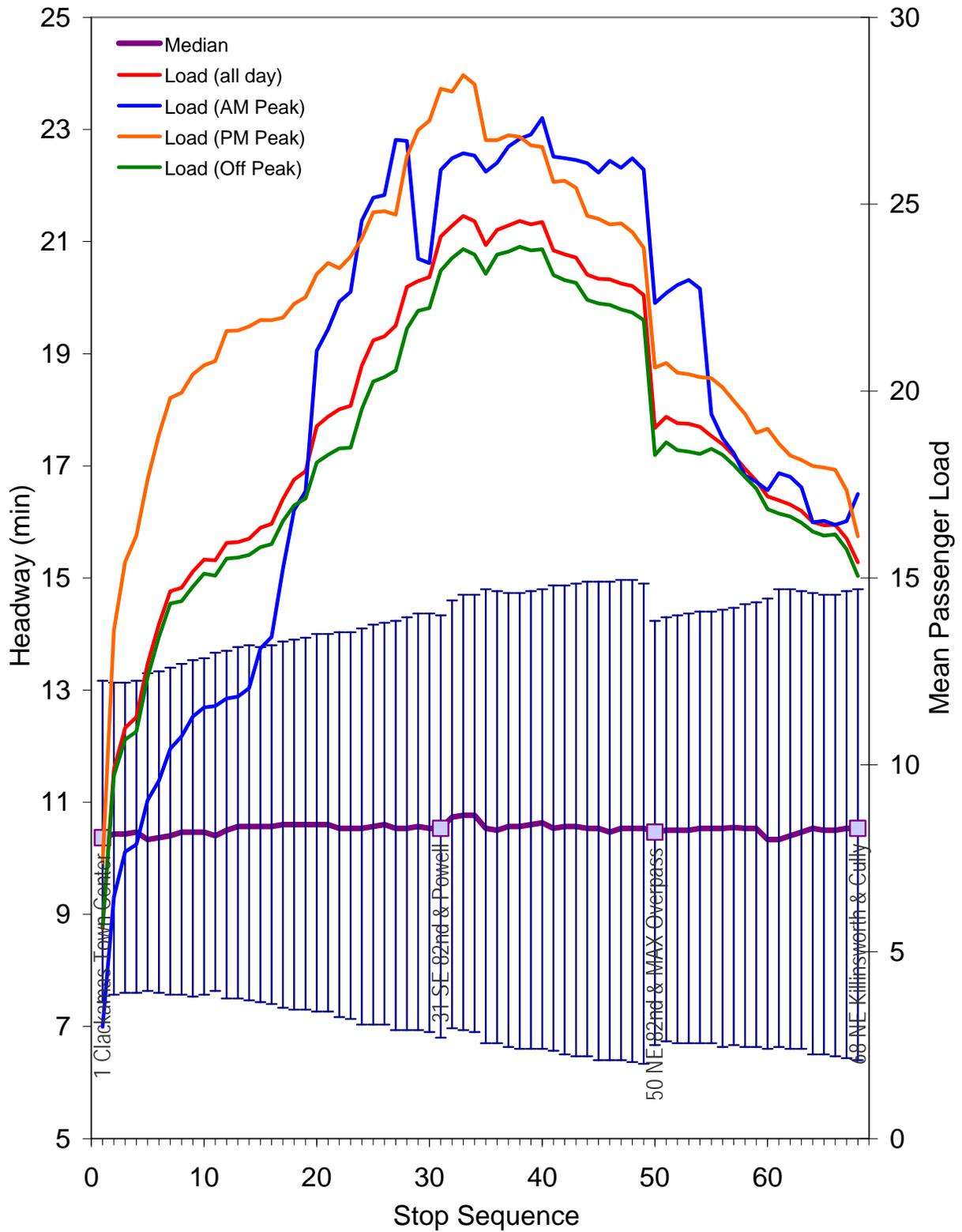
FIGURE 7 Mean and variation of headway and passenger load along route 72 (2007).
