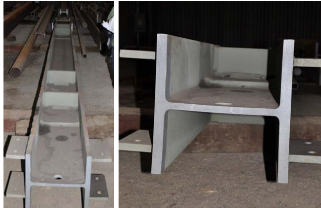
Figure 3.1: Prequalified beam-to-column connection in 65 ksi (450 MPa) W-shape
