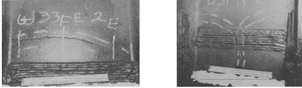
(a) Crack originating at groove weld termination (b) Crack originating at groove weld
