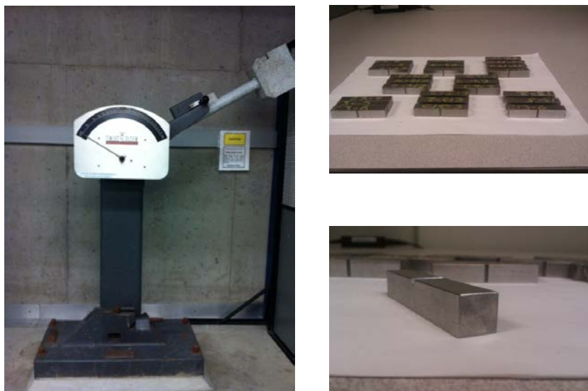
Figure 3.7: CVN specimens and equipment
