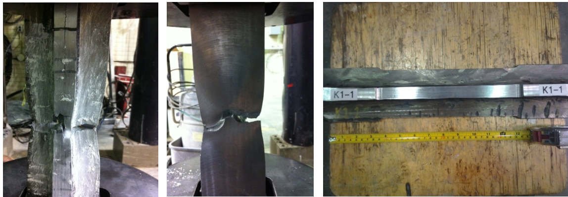
(b) K11 specimen fracture (near the weld)
