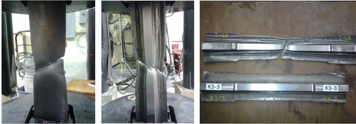
(a) K31 & K33 specimen fracture (away from the weld)
