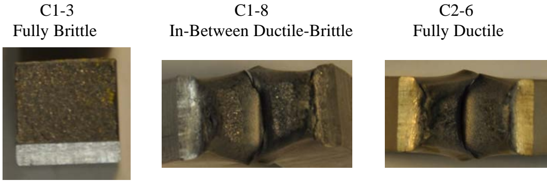
(a) Fracture surfaces for fully brittle, fully ductile and partly brittle-ductile specimen
