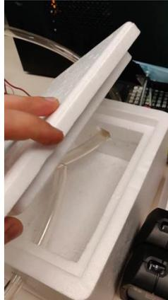
*Figure 40 The ends of the tubes are inserted in the ice box. Cool air is drawn from the box and warm air flows into the box increasing the temperature of the ice.*
