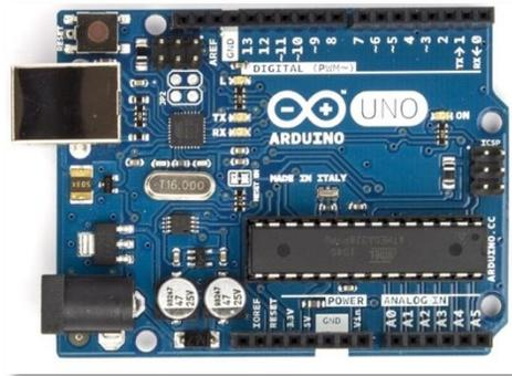
Figure 38 An Arduino Uno device is a powerful microcontroller device commonly sourced from commercial retailers. In our device the microcontroller is used to control the LED array, trigger the camera, and power the fans colling the camera
