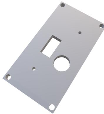
Figure 27 3D render of the lid for the camera holding assembly.
