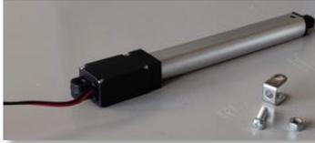
Figure 34 The Linear Actuator helps support the top 3D printed piece and is additionally used for adjusting and leveling the top half.
