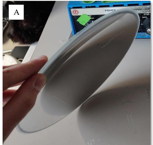
Figure 15 View of the Dome (Parabolic reflector) from the side (A) and top view (B & C)
