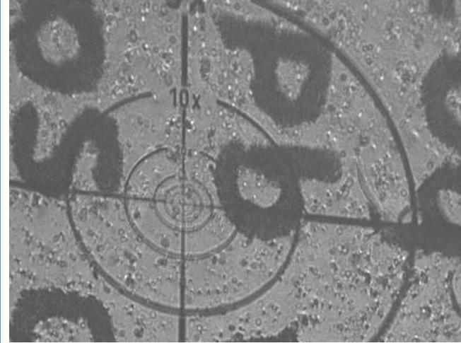
Figure 50 Printed 3pt font letters with a circular scale slide. The slide with the circular target is placed above the translucent film with the letters printed on it. The letters help in locating the slide and for focusing as they provide a course target for initial focus. The slide serves to aid for finer focus and precision measurements.
