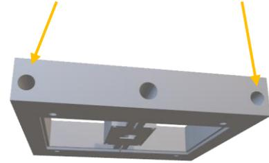
*Figure 30 2 holes on the sides of the frame (gold arrows) allow for optical metal rods to be inserted. The metal rods attach the piece to the rest of the components.*
