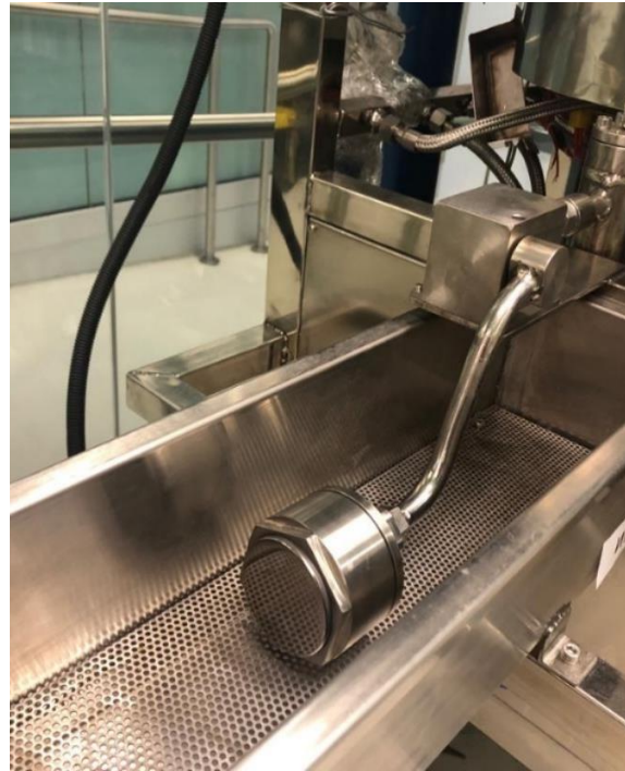
Spinneret head with 300 of 70 \mu\text{m} holes
