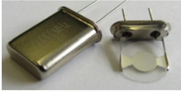
Fig. 1.6 A commercial quartz crystal with the cap on the left and without the cap on the right [20].
