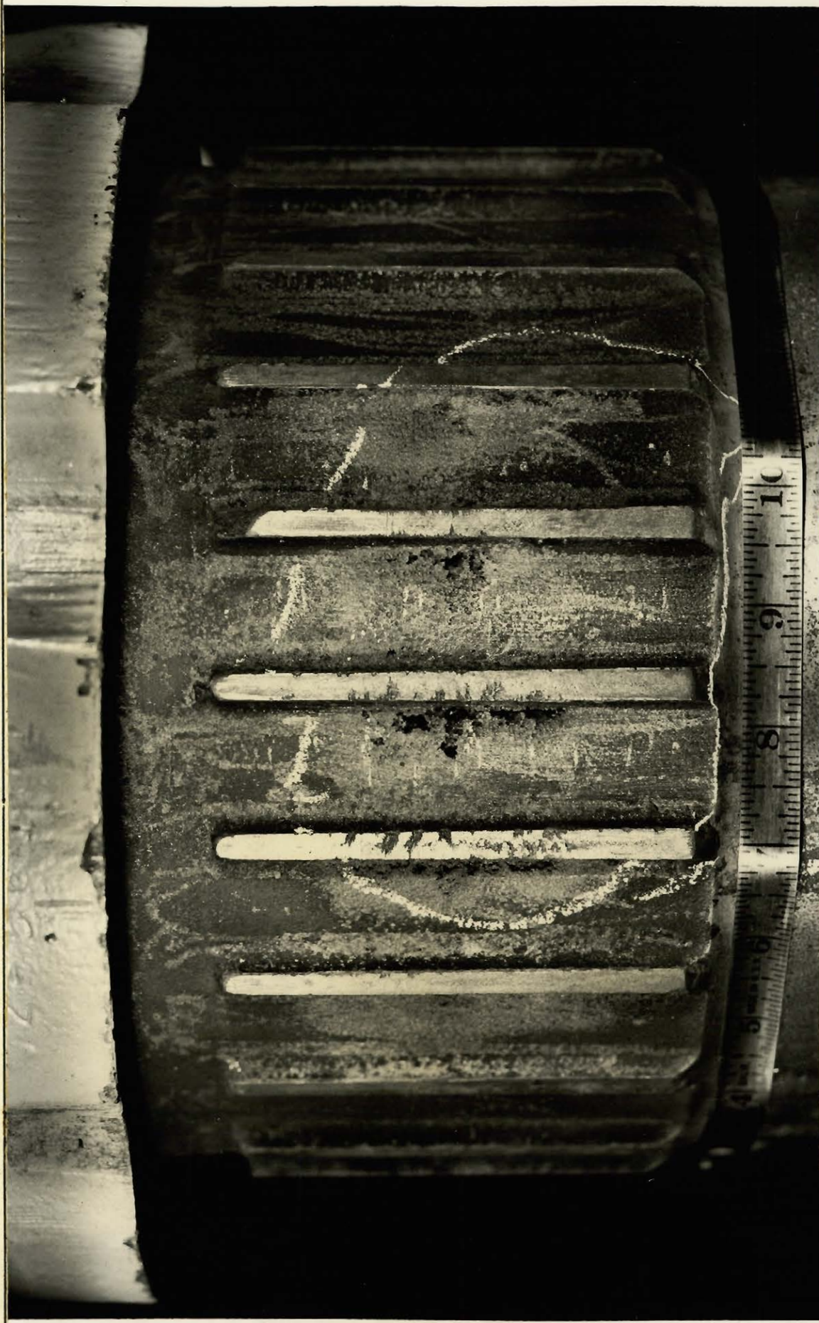
CAVITATED CYLINDER LINER
