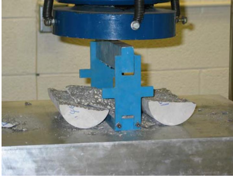
Figure 2-8 - Specimen failing under Splitting Tension Test (Li, 2004)
