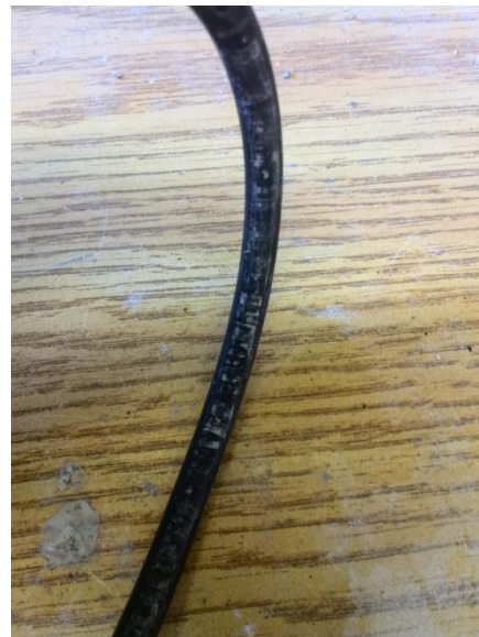
Figure 3-6 - O-Ring damaged after Test
