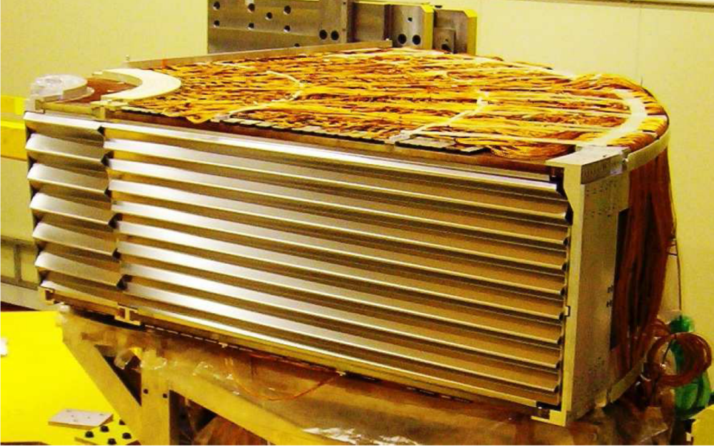
Figure 4.9: A side view of the electromagnetic end-cap calorimeter module [31]. The accordion of the absorbers can be seen.
