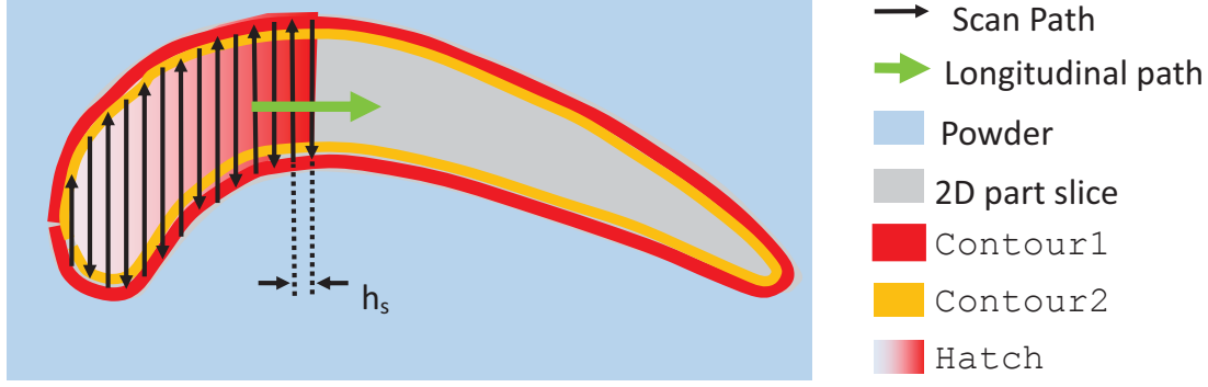
Figure 2-44: Schematic diagram of scan paths used during Hatch melt with longitudinal path along +x direction, and hatch spacing h_s
