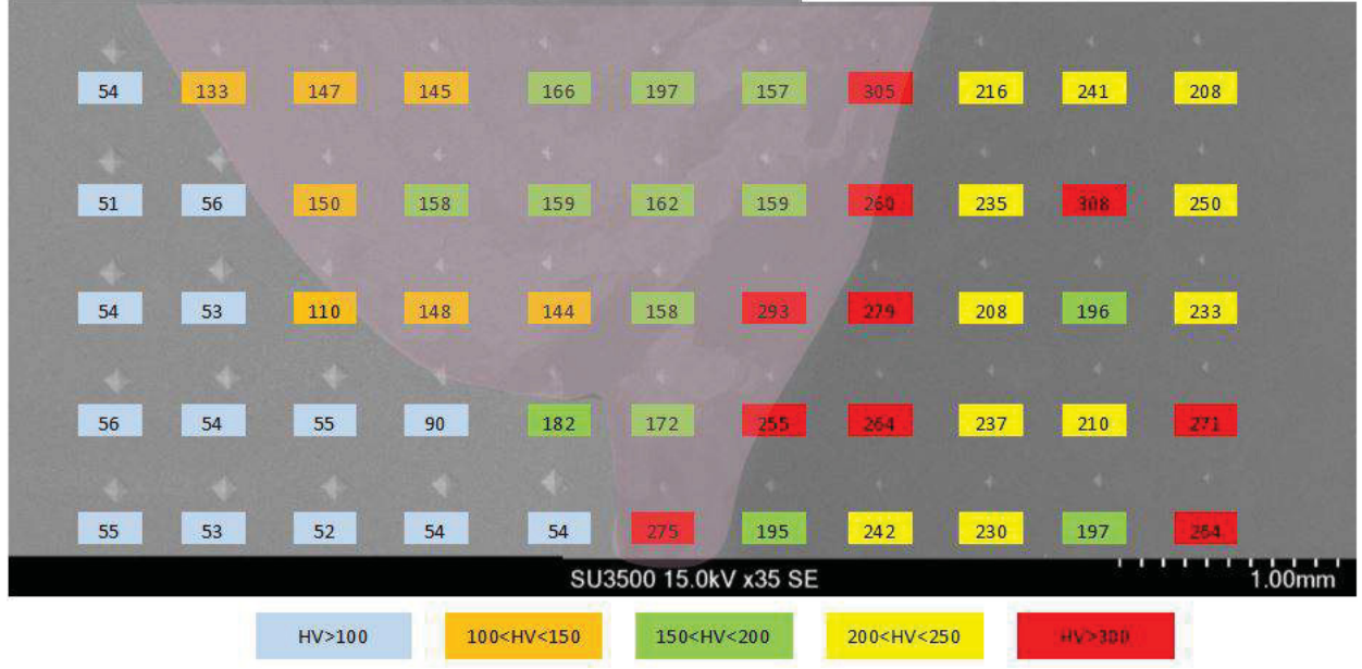
Figure 5–10: Vickers hardness mapping of butt joint formed from Q_l = 224 \text{ J mm}^{-1} , v = 8.6 \text{ mm s}^{-1} and V_{acc} = 110 \text{ kV} and [offset] = 1.0 \text{ mm} . The Nb base metal is on the left, the Ti base metal on the right, and the FZ is delineated by the rose colored outline. Vickers hardness measurements were conducted with a 500gf load and 25s hold.
