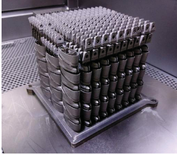
Figure 1–2: Example of nested and stacked build using EB-PBF. Parts were built from Ti64 powder using Arcam hardware. Image provided with permission, courtesy of Metron Advanced Engineering
