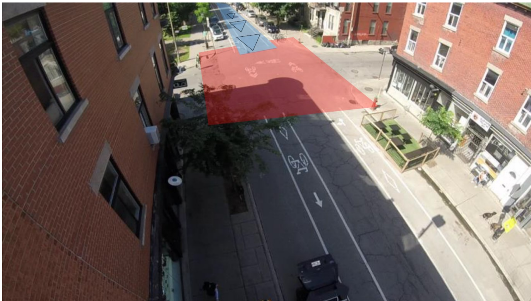
b) Site A-2 Clark-PrinceArthur: Pedestrian crossing at intersection Rue Clark and Rue Prince-Arthur. The pedestrian crossing is on Rue Prince-Arthur, a one-way and one lane-street with a conventional and contraflow bike lanes.
