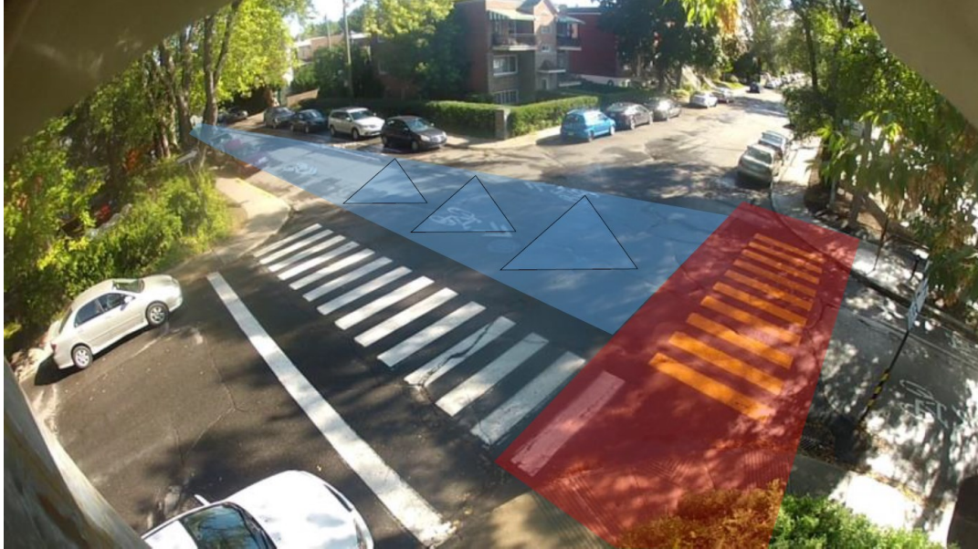
a) Site B-1 Prieur-DeLaRoche: Crosswalk located at the intersection of Rue Prieur and Rue De La Roche. The crosswalk crossing is on Rue Prieur, a one-way and one-lane bike shared street with a contraflow bike lane.
