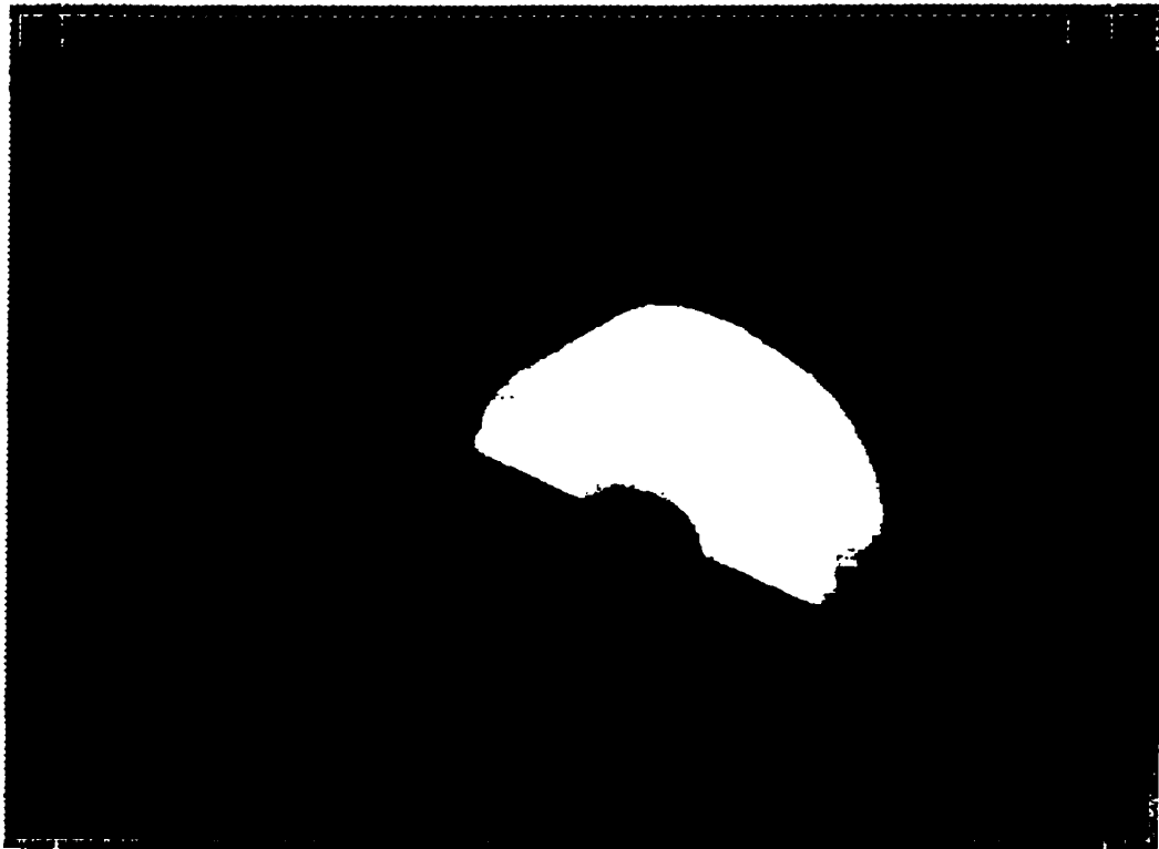
FIGURE 4.6. The presence of random noise in the thresholded image
