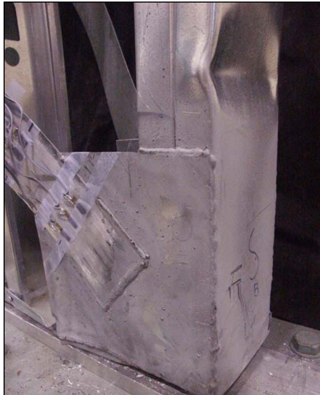
Figure 39: Local buckling of the chord studs due to corner rotation in specimen 4A-C
