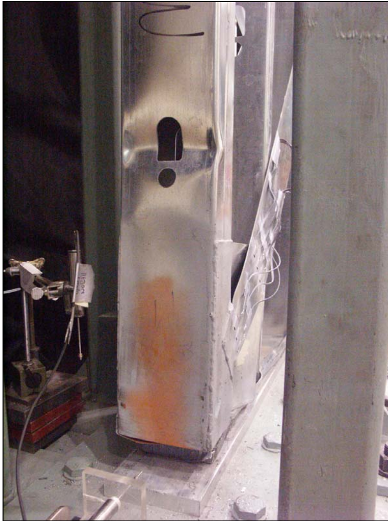
Figure 44: Punching shear failure of the track and local buckling in the chord studs of specimen 5A-M
