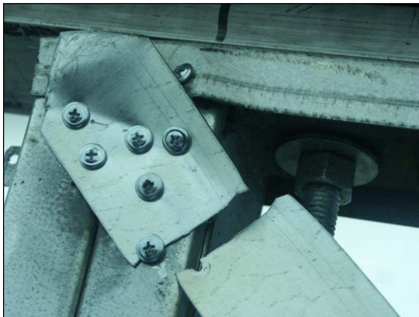
Figure 30: Net cross-section fracture of strap brace in specimen 1A-M
