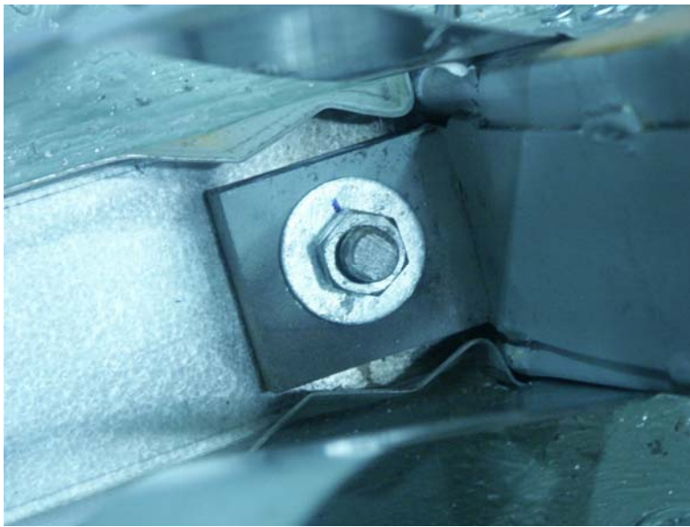
Figure 86: Compression failure in bottom track (overhead view) : Specimen 2B-C
