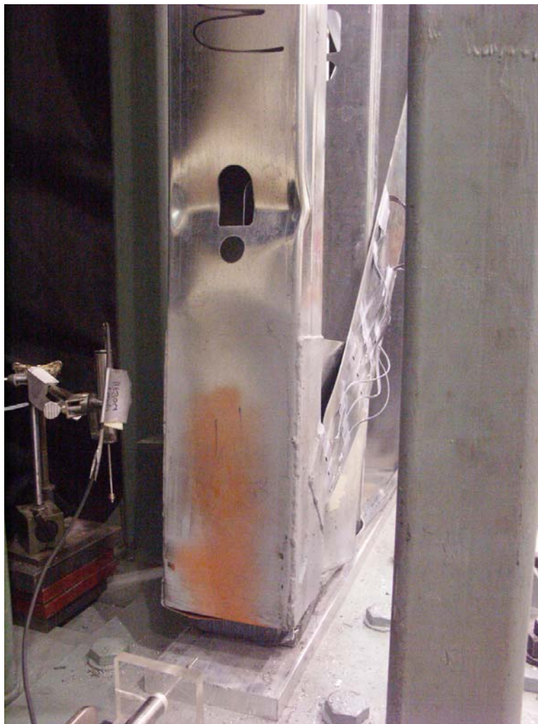
Figure 102: Local buckling of chord studs : Specimen 5A-M
