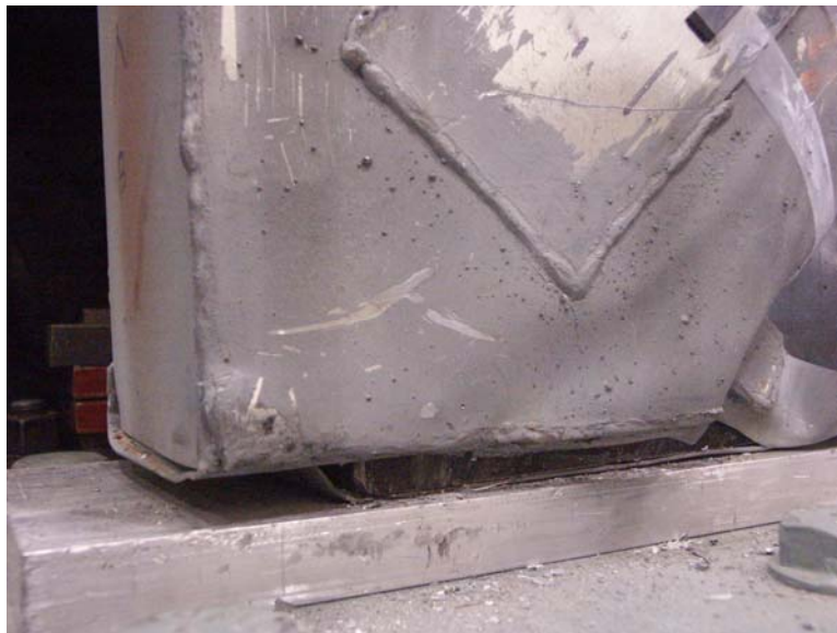
Figure 95: Punching / shear failure of bottom track : Specimen 4A-C
