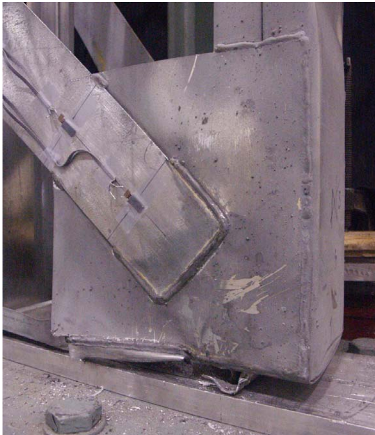
Figure 100: Punching / shear failure of bottom track : Specimen 4C-C
