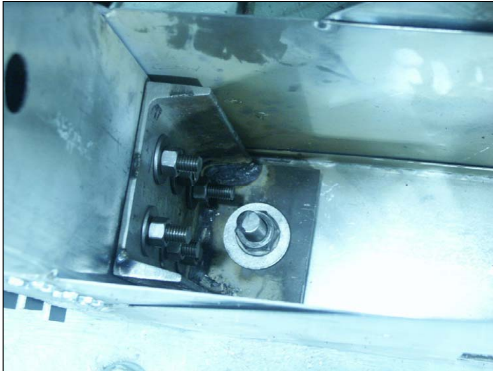
Figure 16: Special holddown for wall specimen 5C-M
