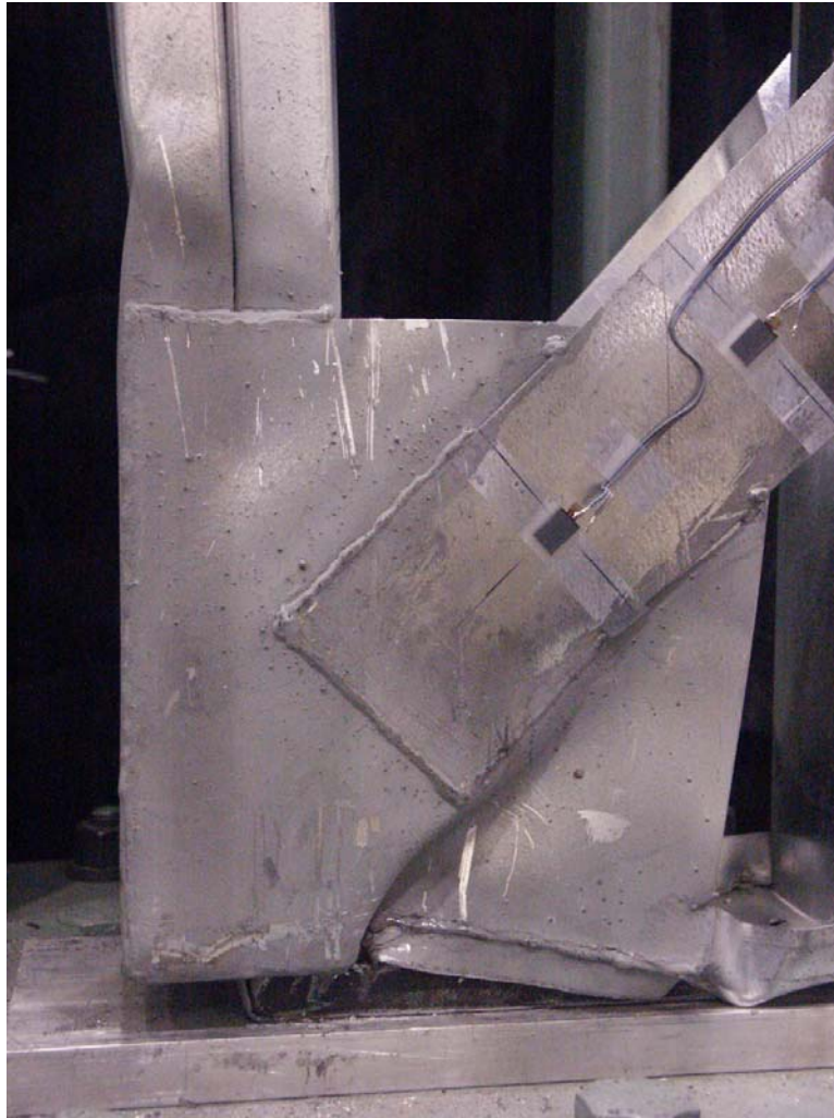
Figure 96: Punching / shear failure of bottom track with compression damage to gusset plate : Specimen 4B-C
