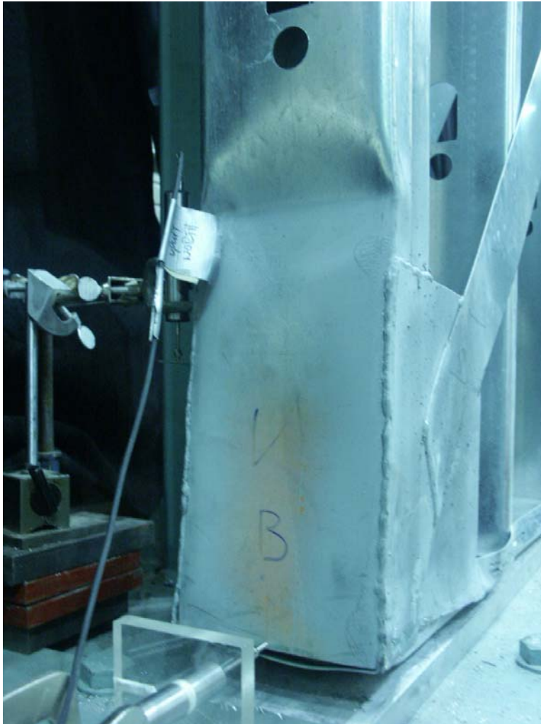
Figure 91: Local buckling of chord studs : Specimen 3C-M
