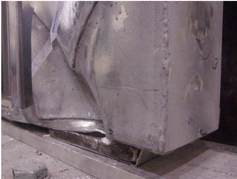
Figure 106: Punching / shear failure of bottom track : Specimen 6B-C
