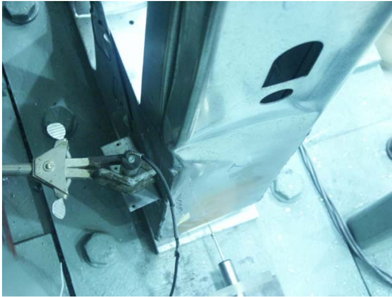
Figure 90: Local buckling of chord studs : Specimen 3B-M
