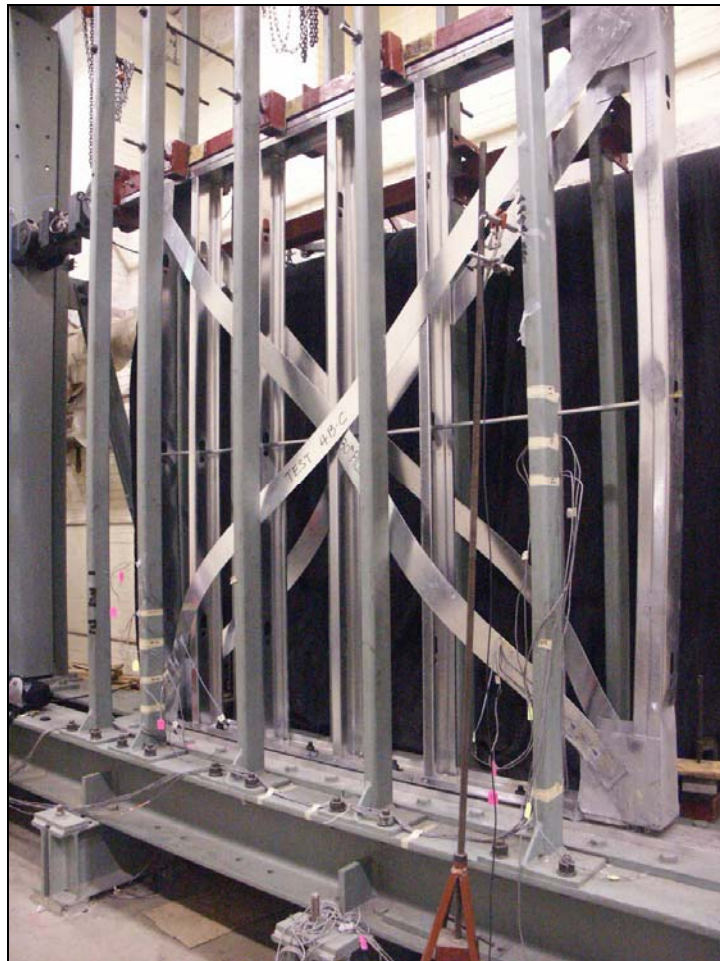
Figure 35: Typical wall with 101 mm (4") strap braces after reversed cyclic testing
