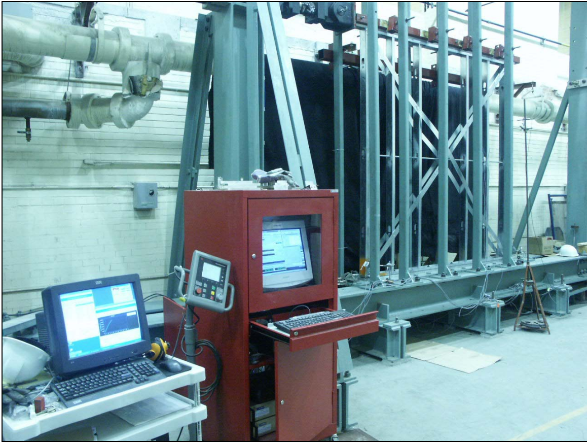
Figure 2: Strap braced wall specimen in test frame
