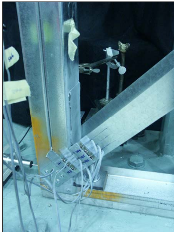
Figure 7: Holddown detail of specimens 1A-M, 1B-M, 1C-M, 2A-C, 2B-C and 2C-C
