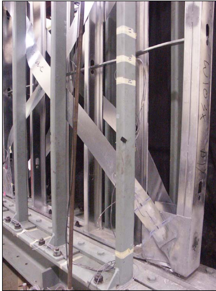
Figure 42: Magnified view of wall with 152 mm (6'') strap braces after reversed cyclic testing
