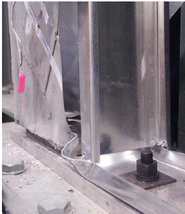
Figure 108: Punching / shear failure of bottom track with uplift of interior studs : Specimen 6B-C
