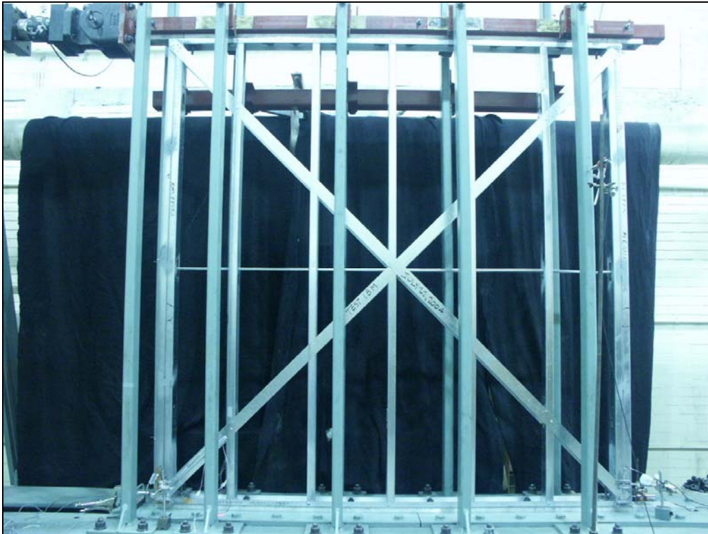
Figure 6: Typical wall with 58.4 mm (2.3'') strap brace prior to testing
