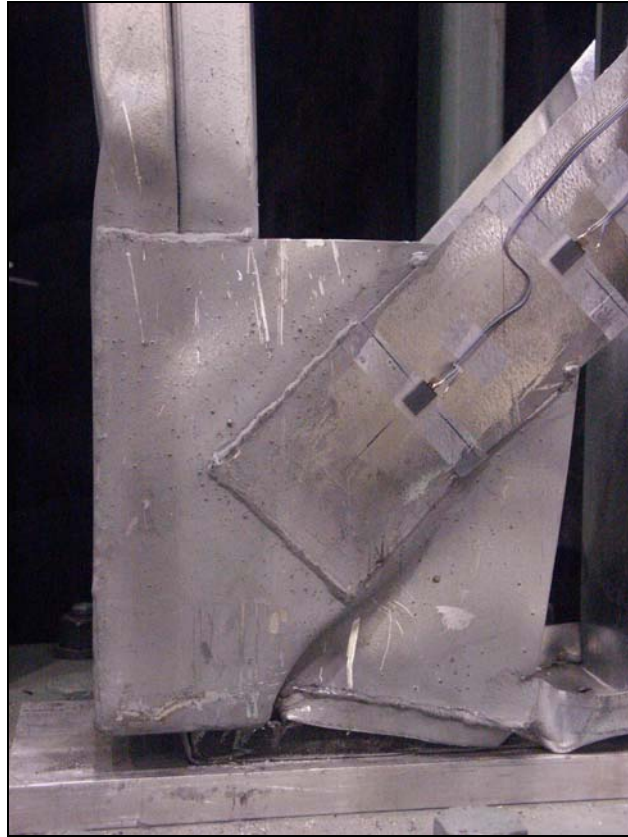
Figure 40: Punching shear failure of the track with compression failure of the gusset plate in specimen 4B-C
