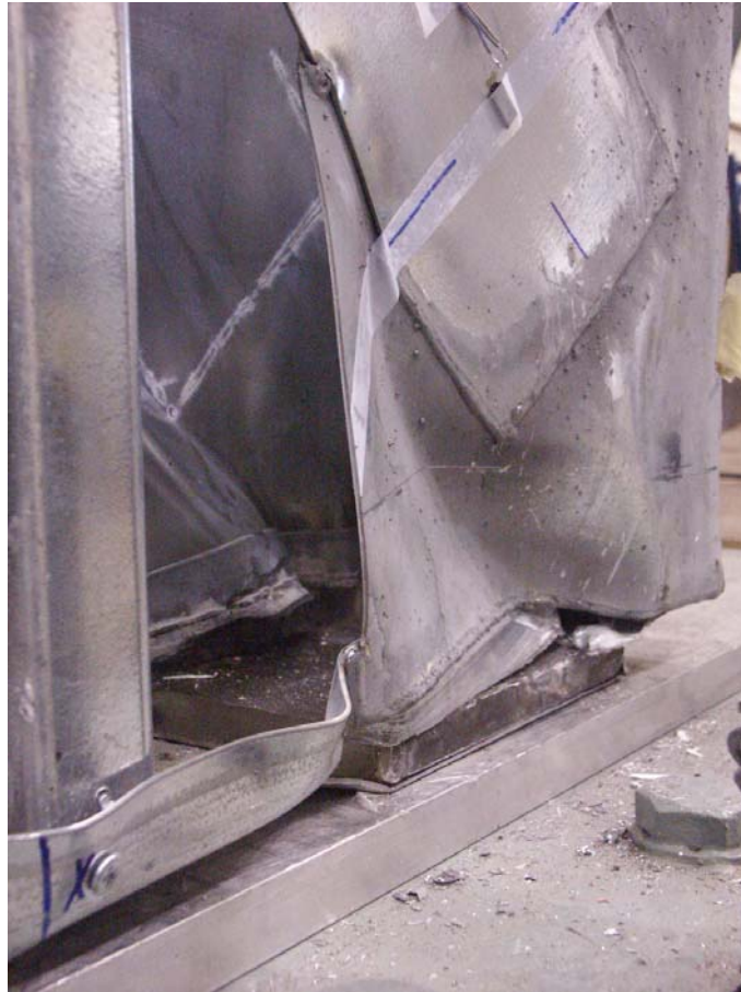
Figure 107: Punching / shear failure of bottom track with compression damage to gusset plate : Specimen 6B-C
