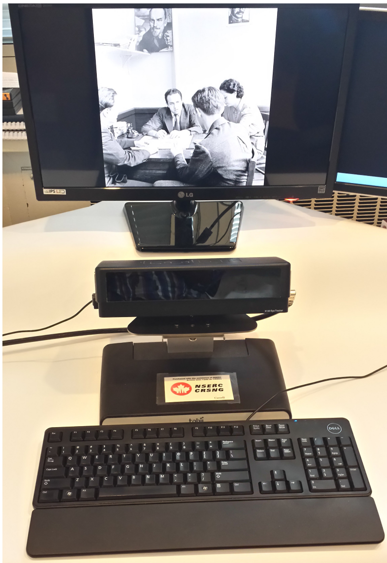
Figure 4-12: Experimental setup using the Tobii X120 eye tracker and the LCD display.
