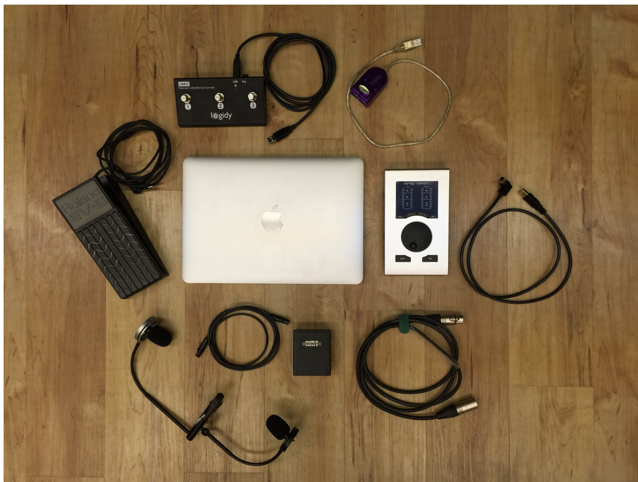
Figure 3.1: A selection of equipment used for the recital. Clockwise from top left: Logidy UM13 Parametric USB MIDI Foot Controller; USB expander hub; RME Babyface Pro audio interface (with USB cable); Digiflex XLR cable; AMT Clarinet double-microphone (with cable and belt pack); Roland EV-5 Expression Pedal. Middle: Macbook Pro 13 inch.
