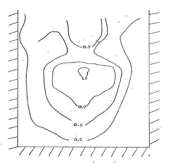
Figure 3.16 Effect of reduced pressure on porosity distribution in an ingot poured at high superheat. Pouring temperature 825°C (1098K), Mould temperature 275°C (548K), Hydrogen concentration 0.14 ml H<sub>2</sub>/100 gm Al (S.T.P:), Pressure over cast 100 torr (13.3KPa).
