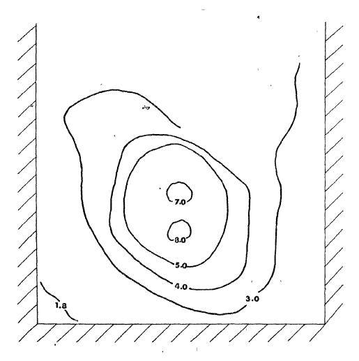
Figure 3.10 Effect of grain refining on porosity distribution in an atmospheric cast ingot poured at high superheat.
