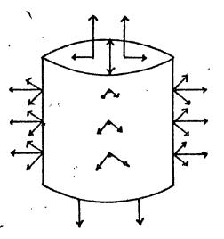
Open topped ingot showing directions of heat loss
