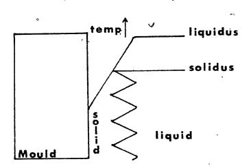
Compared to most metal and alloy systems, Al - 4.5% Cu has a relatively high thermal conductivity which as illustrated in Figure 4.2 results in low temperature gradients that give rise to a large mushy region. As mentioned previously the large mushy region is more difficult to feed, enhancing the possibility of pore formation. As a converse to this, metals displaying a low thermal conductivity allow steep temperature gradients to arise forming a short mushy zone which is easy to feed.
