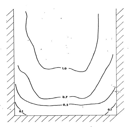
Figure 3.3 Effect of mould temperature on porosity distribution in an atmospheric cast ingot poured at low superheat. Pouring temperature 700°C (973K). Hydrogen Concentration 0.19 ml  $H_2/100$  gm Al (S.T.P.), Mould temperature 70°C (343K).
