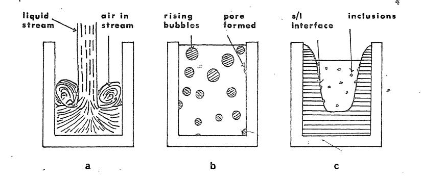
that exist in the melt. This type of pore formation is also possible late in solidification and occurs in the mushy zone; for example, when Al<sub>2</sub>O<sub>3</sub> inclusions are swept out in front of the advancing solid-liquid front.
