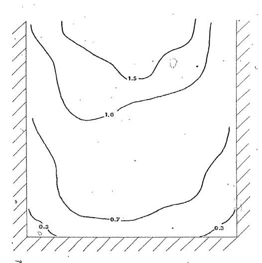
Figure 3.7 Effect of mould temperature on porosity distribution in an atmospheric cast ingot noured at high superheat. Pouring temperature 825°C (1098K).
