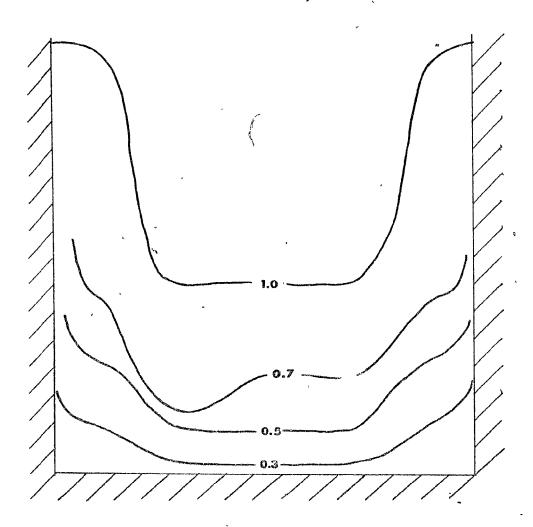
Effect of mould temperature on porosity Figure 3.4 distribution in an atmospheric cast ingot poured at low superheat. Pouring temperature 700°C (973K), Hydrogen Concentration 0.19 ml  $H_2/100$  gm Al (S.T.P.) Mould temperature 240 °C (513K).
