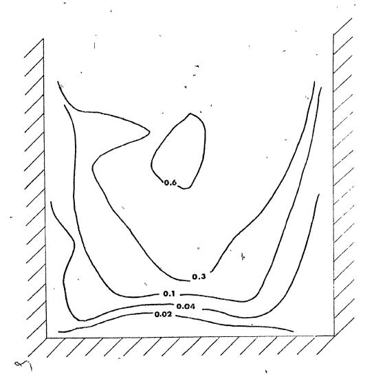
Figure 3.13 Effect of reduced pressure on porosity distribution in a cast ingot poured at low superheat.
