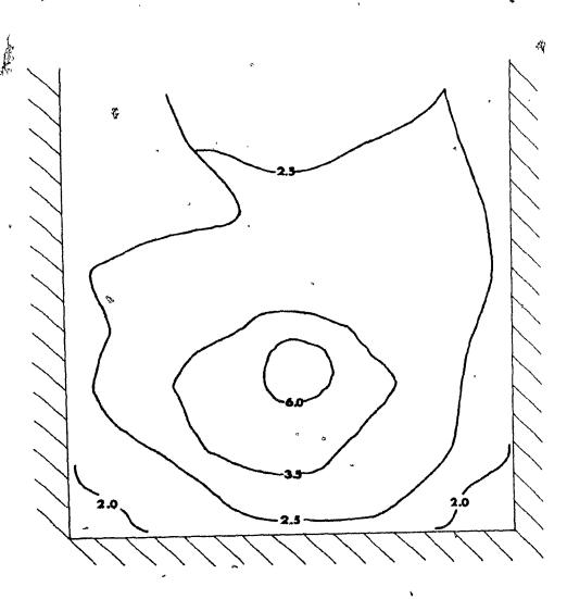
Figure 3.9 Effect of very high superheats on porosity distribution in an atmospheric cast ingot. Pouring temperature 950°C (1223K), Nould temperature 259°C (523K), Hydrogen concentration 0.45 ml H<sub>2</sub>/100 gm Al (S.T.P.).
