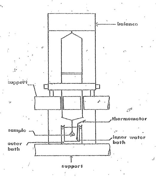
Figure 2.7 Density Apparatus
