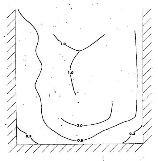
Figure 3.8 Effect of mould temperature on porosity distribution in an atmospheric cast ingot poured at high superheat. Pouring temperature 825°C (1098K), Mould temperature 400°C (673K), Hydrogen concentration 0.46 ml H<sub>2</sub>/100 gm Al (S.T.P.).
