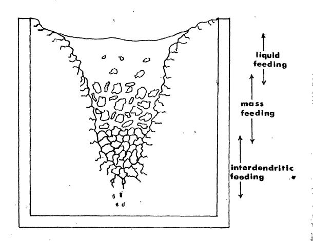
feeding can lead to blocking of feeding channels on the macroscopic scale. This type of feeding must be highly dependant on such variables as the primary dendrite arm spacing and the dimensions of the casting. Mass feeding of grain refined ingots should be easier than feeding of an ingot with long columnar grains, since the flow of liquid metal between smaller equiaxed grains is easier than down long channels between columnar grains.
