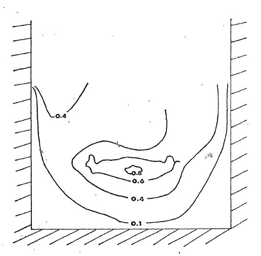
Figure 3.19 Effect of mould temperature on porosity distribution in an ingot poured under reduced pressure. Pour temperature 700°C (973K), Hydrogen concentration 0.02 ml H<sub>2</sub>/100 gm Al (S.T.P.). Pressure over cast 0.20 torr (26.6Pa), Nould temperature 525°C (798K), Mean porosity 0.5%.
