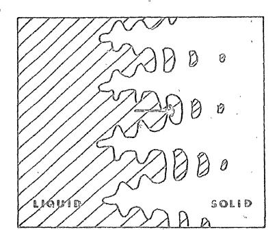
Figure 1.11 Schematic of Solid Feeding (12,21).
