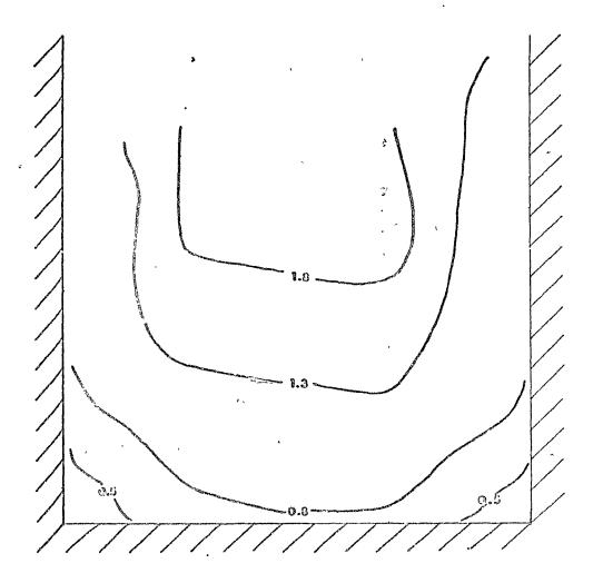
increased, ie. 1.0% at 250°C (523K) and 2.9° at 400°C (673K). The extreme case occured when the pouring temperature was increased to 950°C (1223K) with a 250°C (523K) mould temperature. The distribution then was such that porosity was concentric about the centre of the ingot (Figure 3.9); the same pattern as exhibited in Figure 3.8, but with higher centre and mean porosity (Table 3.1).
