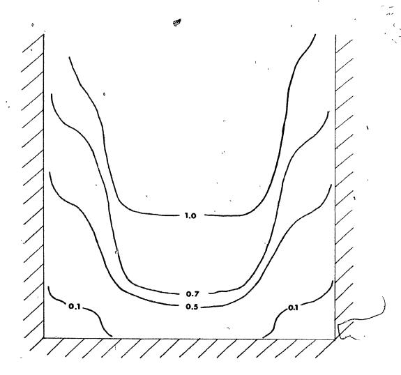
Figure 3.6 Porosity profile of atmospheric cast ingot poured at a higher superheat. Pouring temperature 825°C (1098K), Mould temperature 25°C (298K), Hydrogen concentation 0.46 ml H<sub>2</sub>/100 gm Al (S.T.P.).
