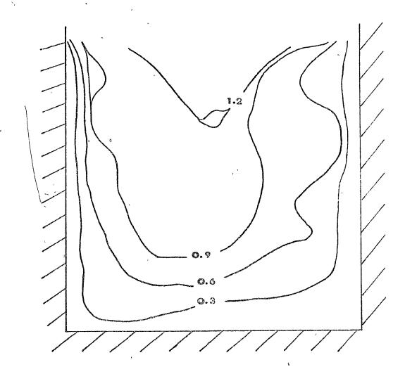
Figure 3.15 Effect of pressure on porosity distribution. Pouring temperature 700°C (973K), Nould temperature 280°C (553K), Hydrogen concentration 0.03 ml H<sub>2</sub>/100 gm Al (S.T.P.) Pressure over cast 760 torr (101.3 KPa), Mean porosity 0.5%.
