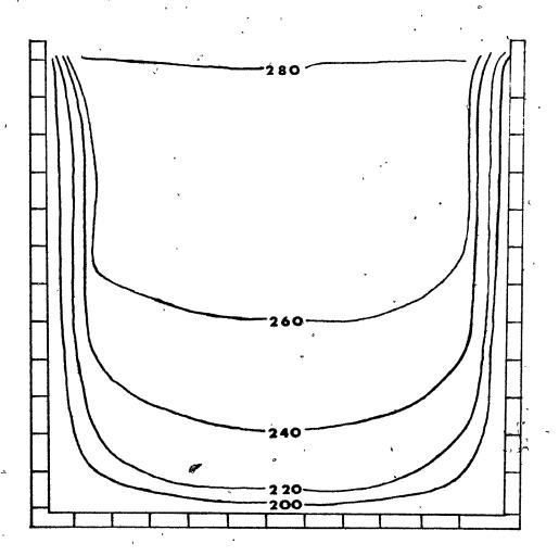
Figure 3.35 Local Solidification Time as a function of position in the mould. Pouring temperature 950°C (1223K), Mould temperature 25°C (298K).
