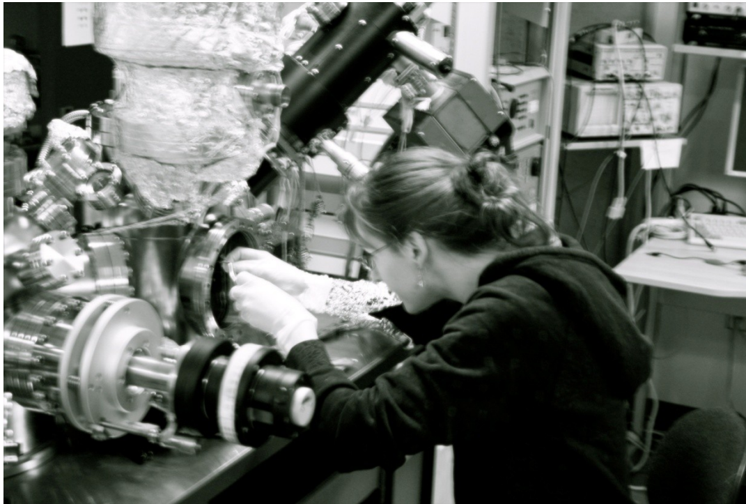
Figure H4: Lily's Photograph of Herself Fixing a Tip on the Scanning Tunneling Microscope
