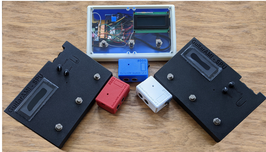
Fig. 4.25 Three sets of the GuitarAMI consisting of the main module and remote sensor (Reproduced with permission).
