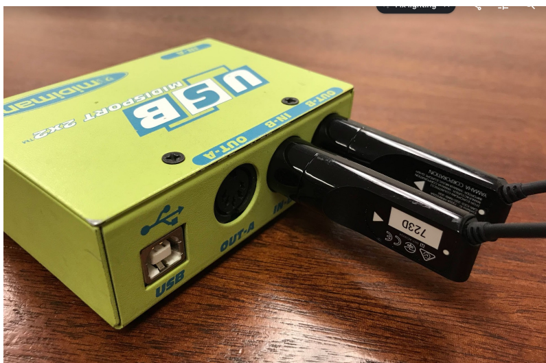
Fig. 4.13 The Yamaha MD-BT01 connected to a M-Audio MIDISport 2x2 USB-MIDI interface.
