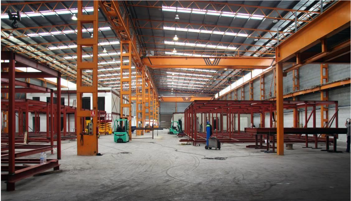
Figure 3.15 Interior view of Gava's factory. In the image, several projects under different stages of prefabrication are seen. On the far left it is possible to visualize how the stacked modules used to check dimensions and manufacturing details before they land on the rooftop. May 30, 2018
