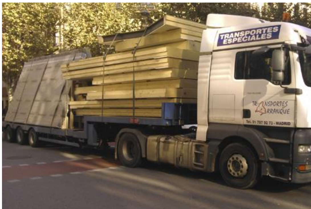
Figure 3.27 Wooden panels fabricated by Novadomus.. Source LCT (Enric Granados 69, Clase Energética A, 2015)
