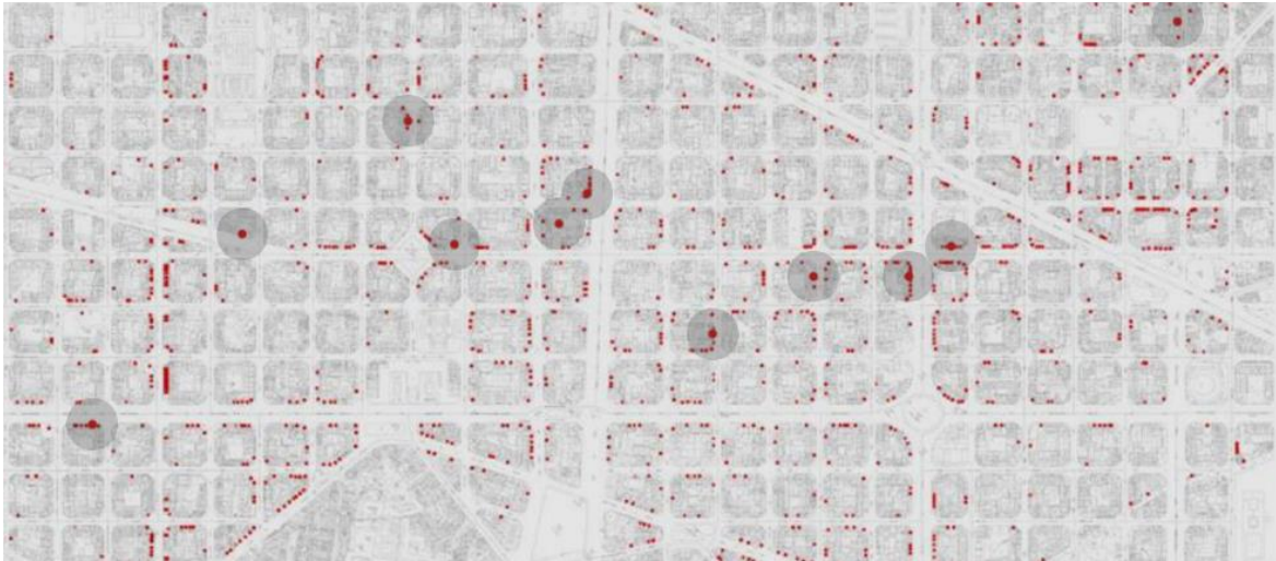
Figure 3.3 LCT's 'rooftop-lost-space' map in Barcelona's Eixample. The red dots represent the buildings with remaining buildable space, and the outlined dots represent the ones already built as of June 6, 2018. Adapted by the author using the base research-map from: (Artés, Wadel, & Martí, Vertical Extension and Improving of Existing Buildings , 2017)
