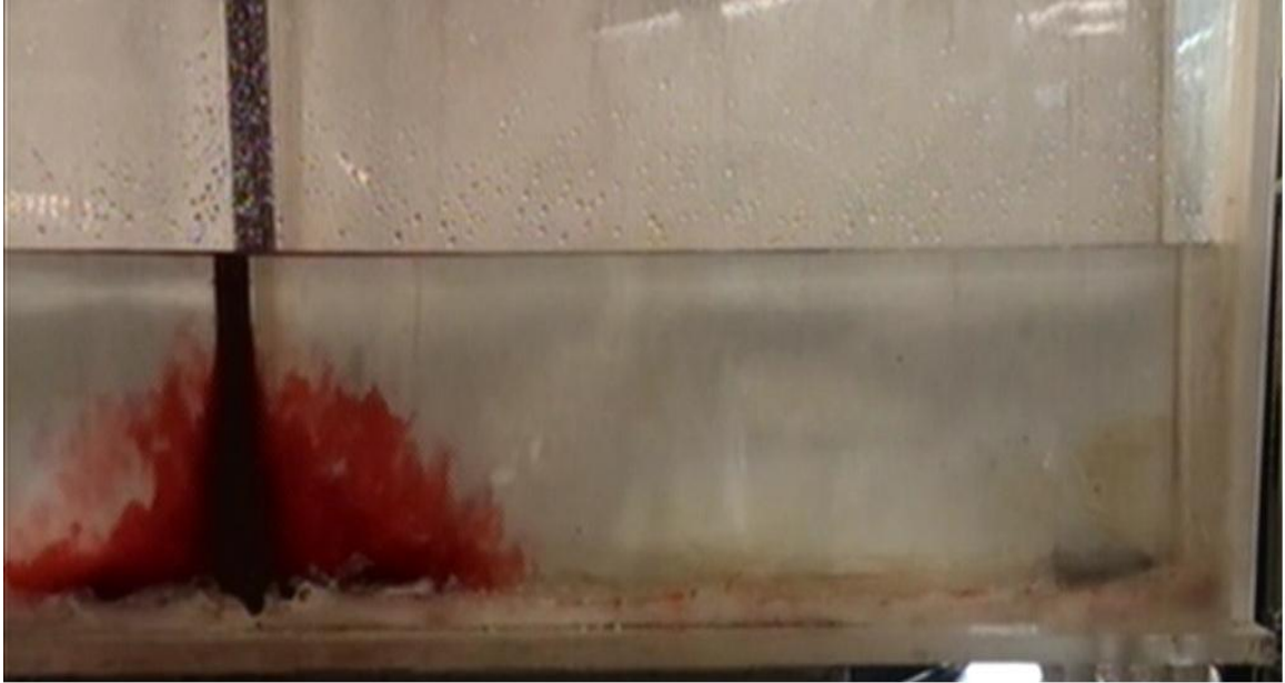
Figure 4.16c. Tracer distribution in the bare tundish arranged with the LS after 5s
