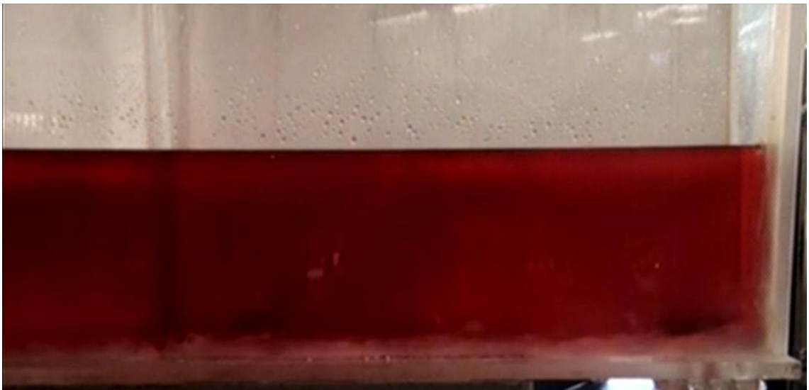
Figure 4.19c. Tracer distribution in the bare tundish arranged with the LS after 120s
