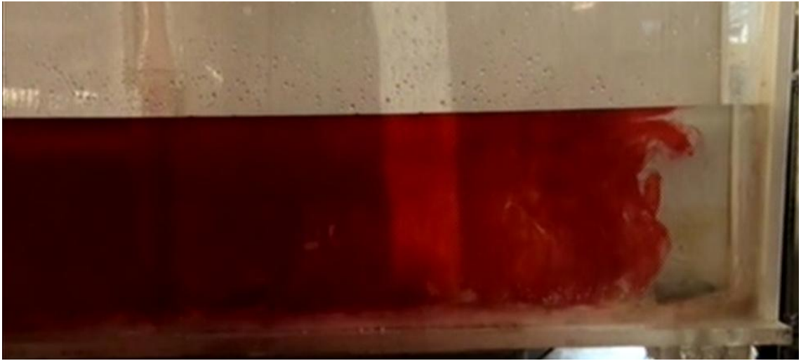
Figure 4.18c. Tracer distribution in the bare tundish arranged with the DLS after 32s
