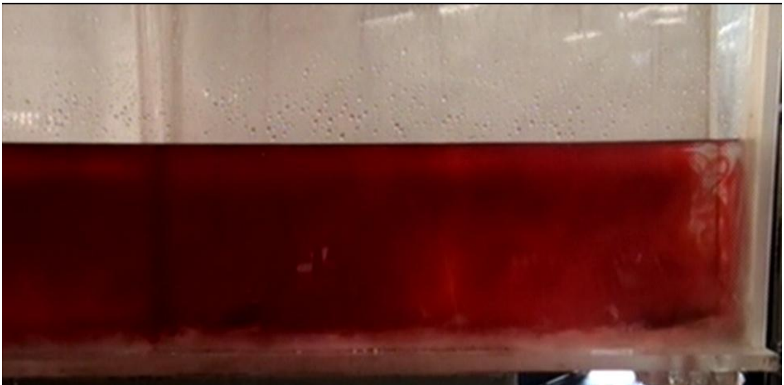
Figure 4.19a. Tracer distribution in the bare tundish arranged with the LS after 60s
