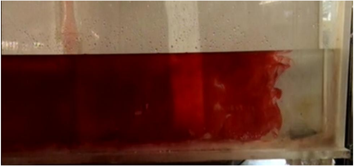
Figure 4.18a. Tracer distribution in the bare tundish arranged with the DLS after 28s
