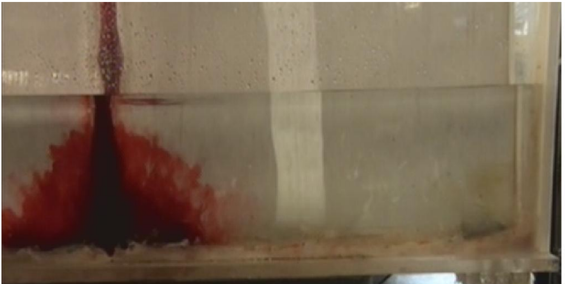
Figure 4.16f. Tracer distribution in the bare tundish arranged with the DLS after 6s
