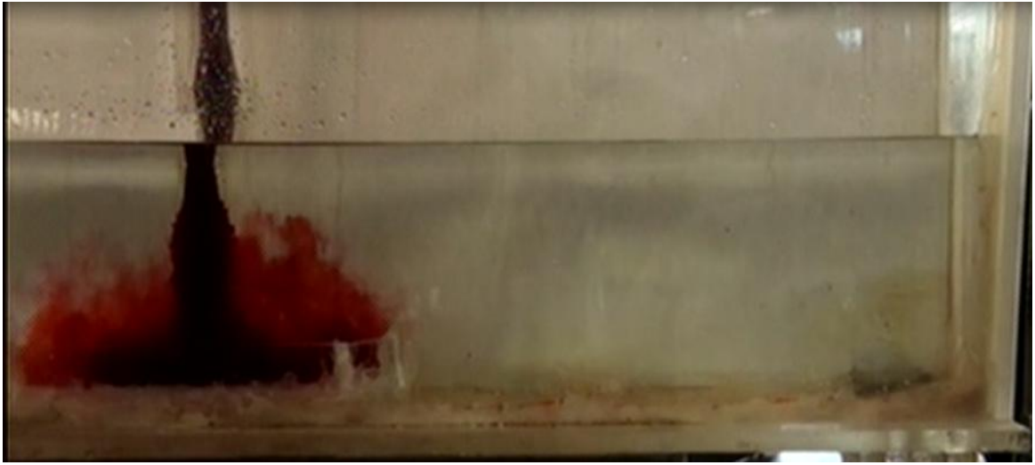
Figure 4.20d. Tracer distribution in tundish, arranged with the DLS and IP, after 5s
