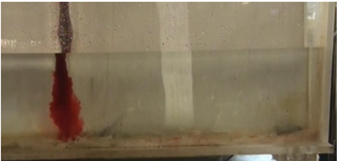
Figure 4.16b. Tracer distribution in the bare tundish arranged with the DLS after
