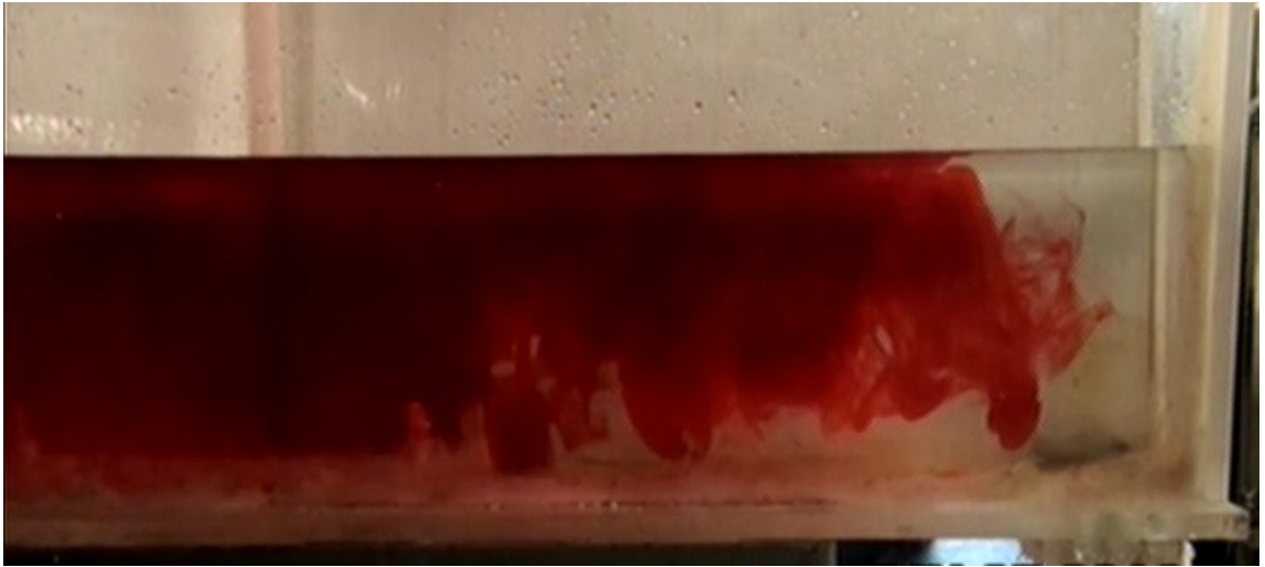
Figure 4.22c. Tracer distribution in tundish, fitted with the LS and IP, after 32s
