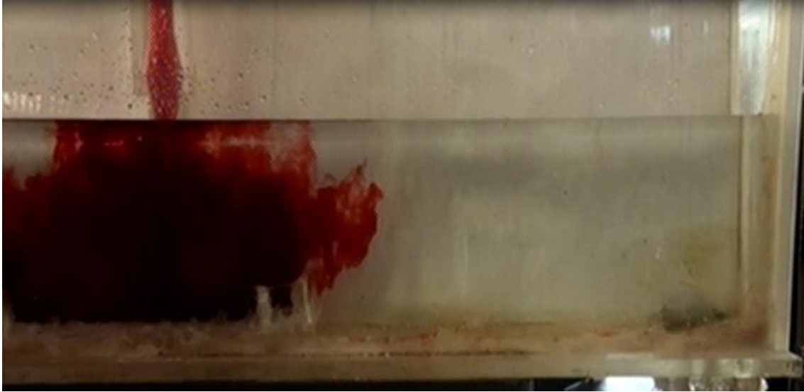
Figure 4.21b. Tracer distribution in tundish arranged with the DLS and IP after 8s
