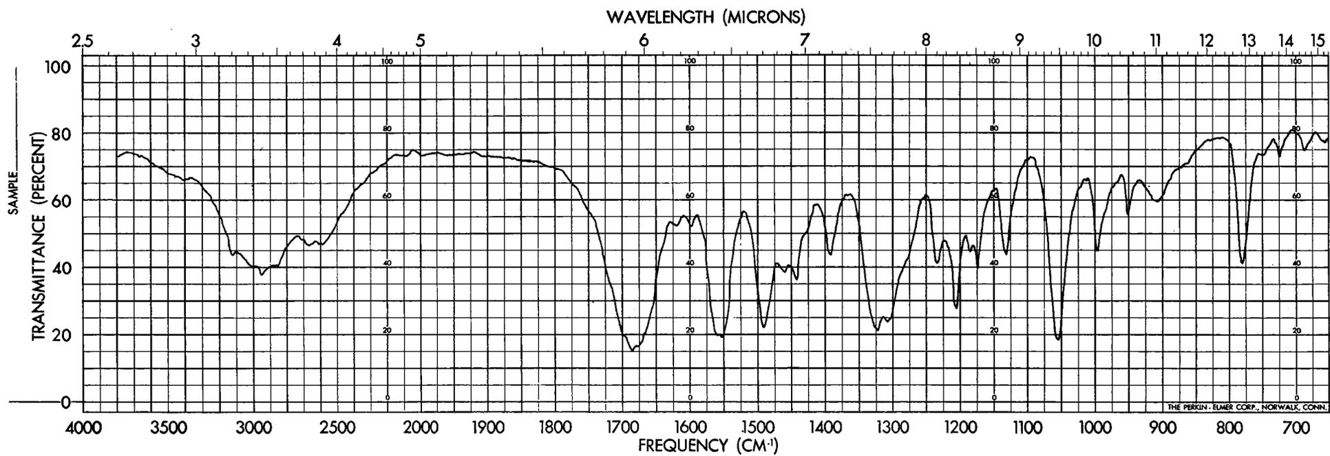
Figure 21. Infrared Absorption Spectrum of 3,4-Dimethoxy-2-Furancarboxylic Acid.
