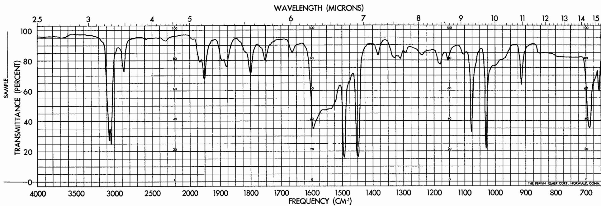
Figure 7. Infrared Absorption Spectrum of Triphenylmethane.
