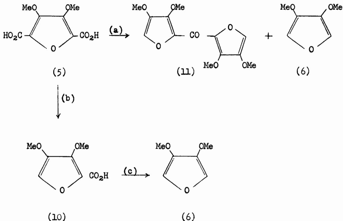
Conditions: (a) strong, fast heating; (b) slow heating; (c) further heating.
