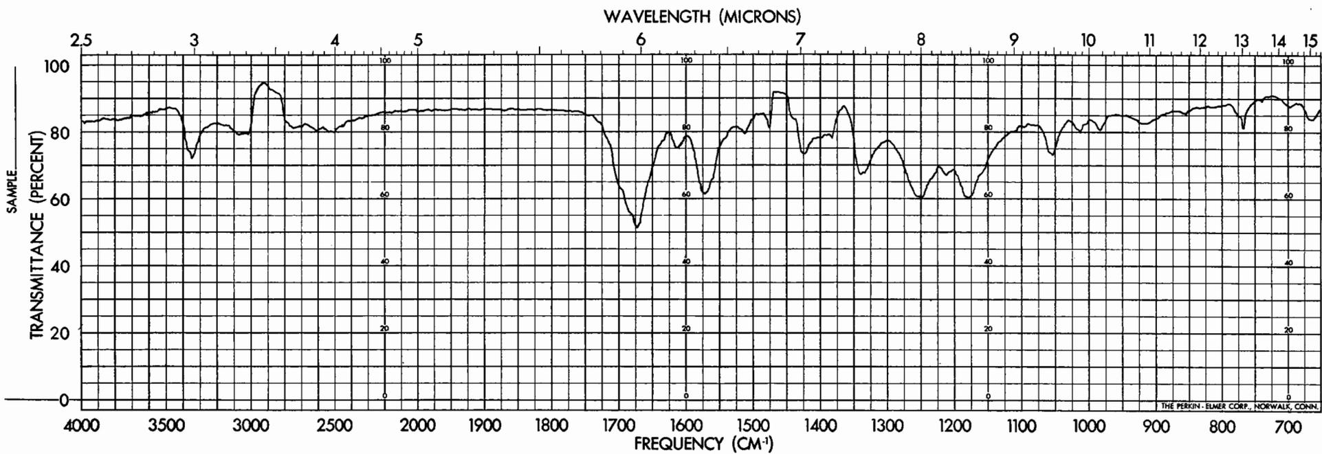
Figure 16. Infrared Absorption Spectrum of Ethyl 5-Carboxy-3-Hydroxy-4-Methoxy-2-Furancarboxylate.
