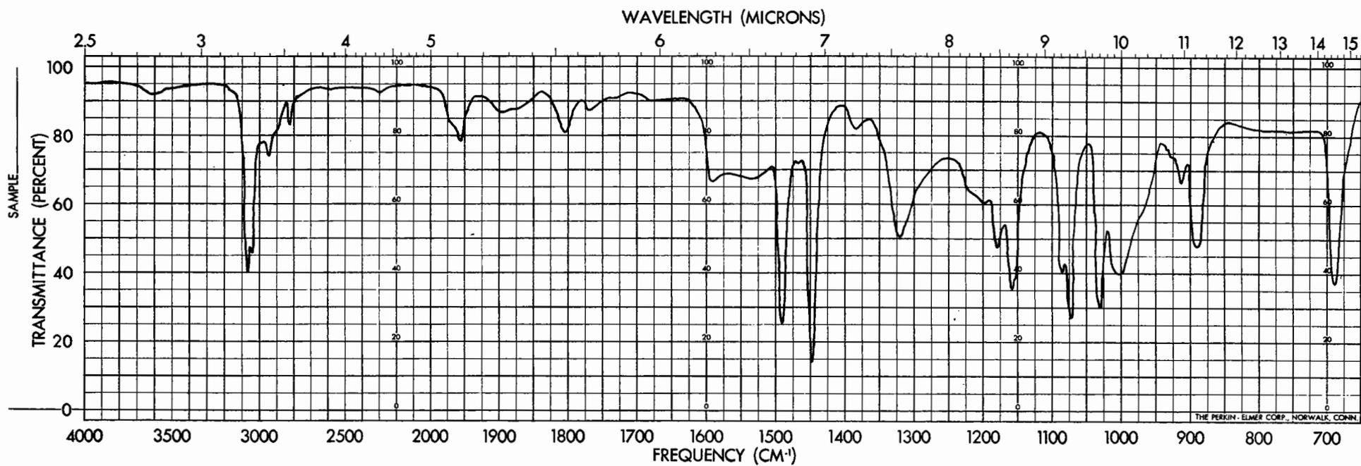
Figure 6. Infrared Absorption Spectrum of Methoxytriphenylmethane.
