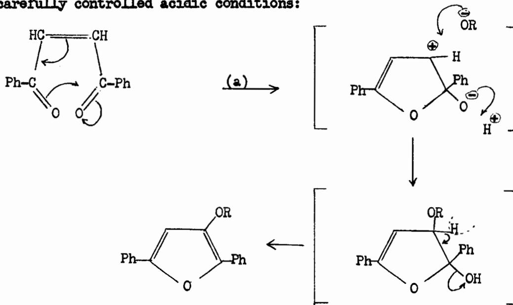
Reagents: (a) ROH +  $\text{R}_3\text{N.HCl}$  (pH 2-3)
