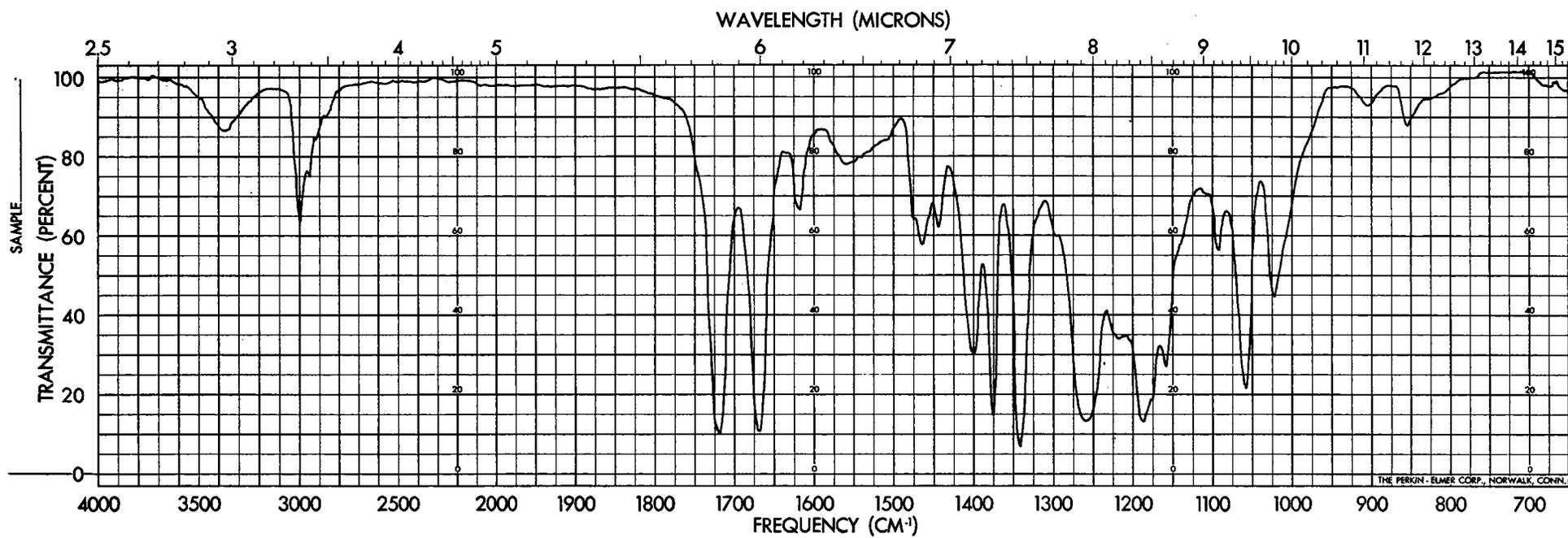
Figure 18. Infrared Absorption Spectrum of Diethyl 3-Hydroxy-4-Methoxy-2,5-Furandicarboxylate.
