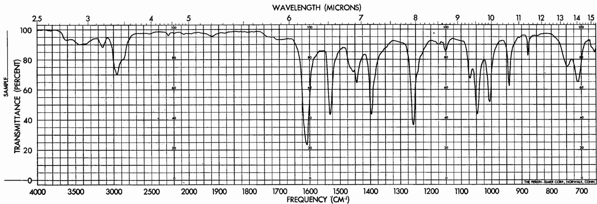
Figure 1. Infrared Absorption Spectrum of 2-Methoxyfuran.
