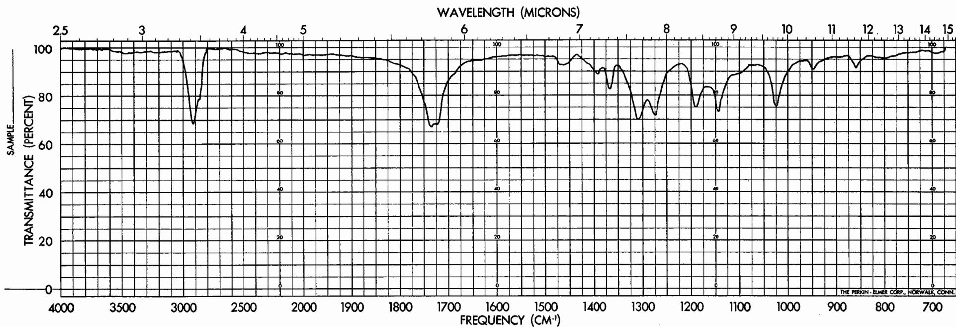
Figure 17. Infrared Absorption Spectrum of Product of Condensation of Diethyl Diglycolate with Diethyl Mesoxylate in the Presence of Potassium *n*-Butoxide.
