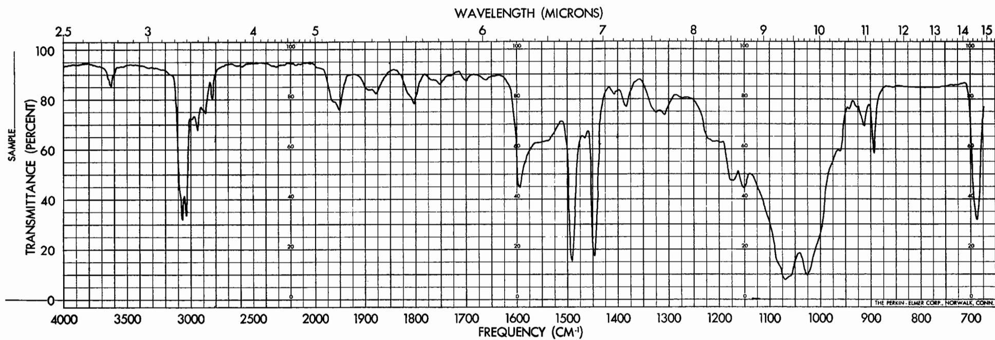
Figure 5. Infrared Absorption Spectrum of Product of Reaction between Triphenylmethylsodium and Dimethyl Peroxide.
