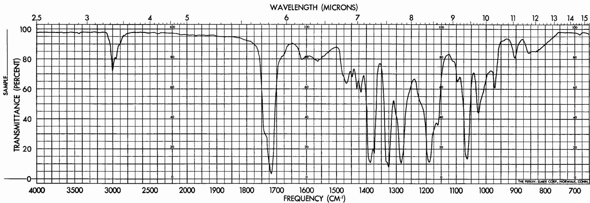
Figure 22. Infrared Absorption Spectrum of Diethyl 3-Methanesulfonyloxy-4-Methoxy-2,5-Furandicarboxylate.
