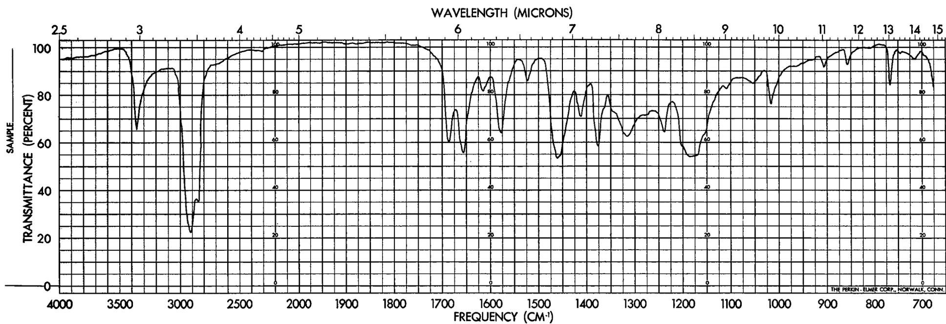
Figure 15. Infrared Absorption Spectrum of Diethyl 3,4-Dihydroxy-2,5-Furandicarboxylate.
