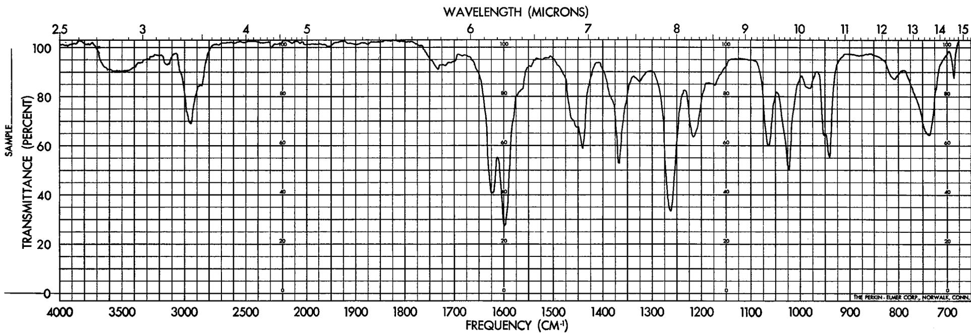
Figure 2. Infrared Absorption Spectrum of 2-Methoxy-5-Methylfuran.
