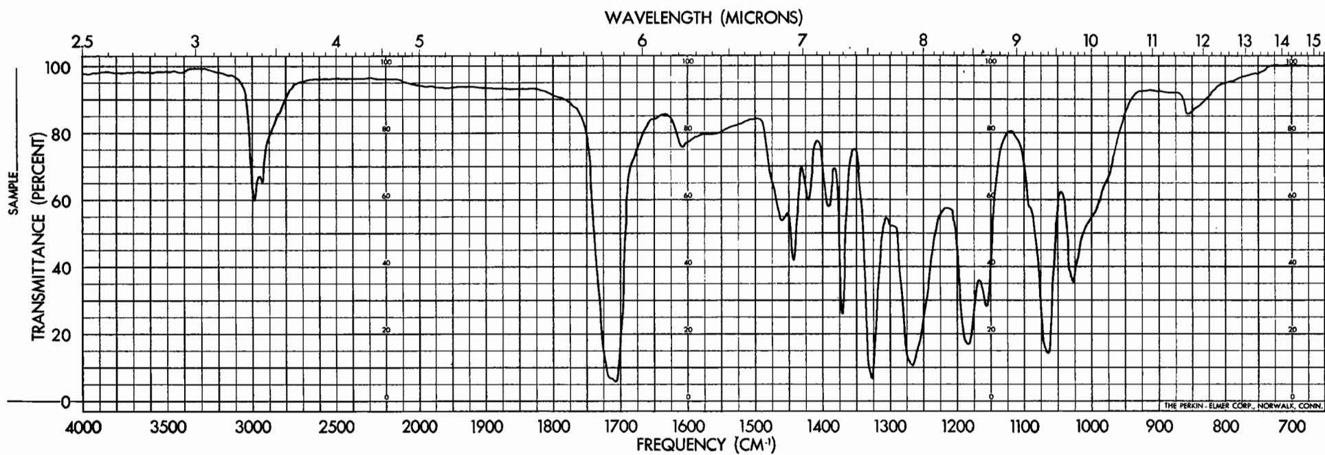
Figure 19. Infrared Absorption Spectrum of Diethyl 3,4-Dimethoxy-2,5-Furandicarboxylate.
