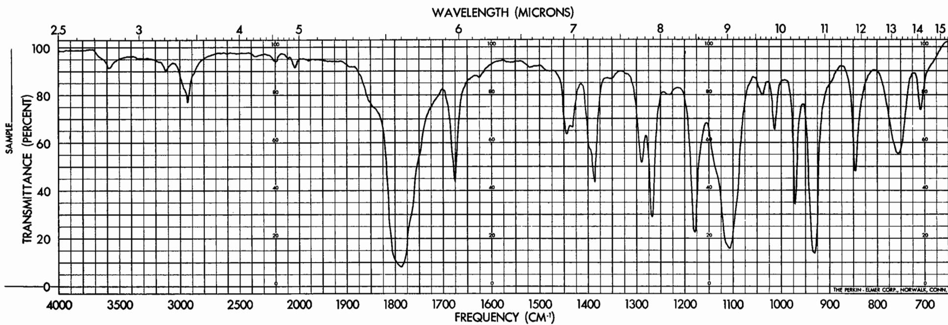
Figure 23. Infrared Absorption Spectrum of  $\alpha$ -Angelica Lactone.
