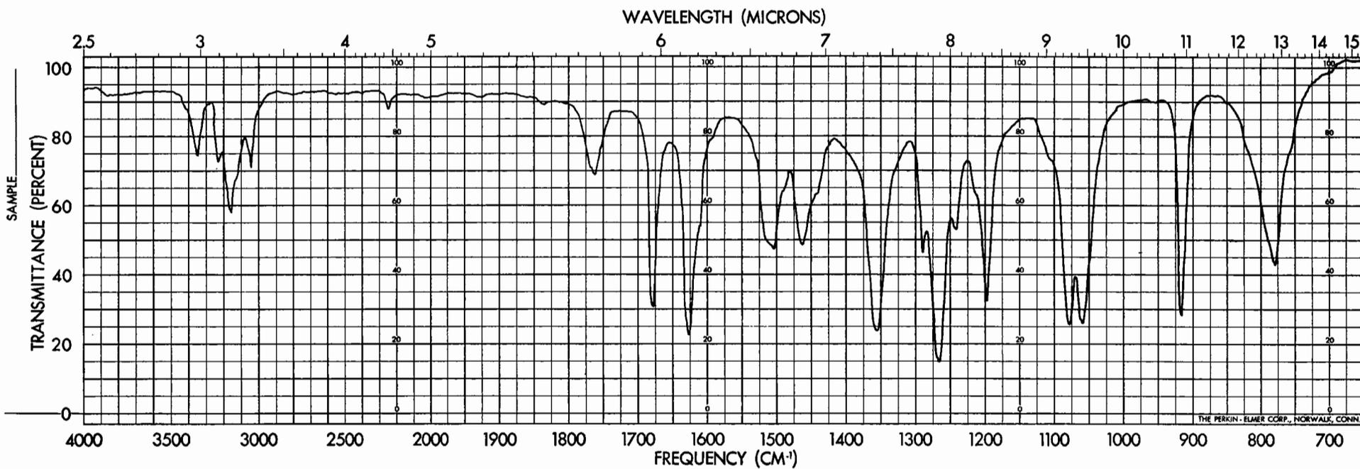
Figure 12. Infrared Absorption Spectrum of Mixture of 3,4-Dimethoxyfuran and Di-2-(3,4-Dimethoxyfuryl) Ketone.
