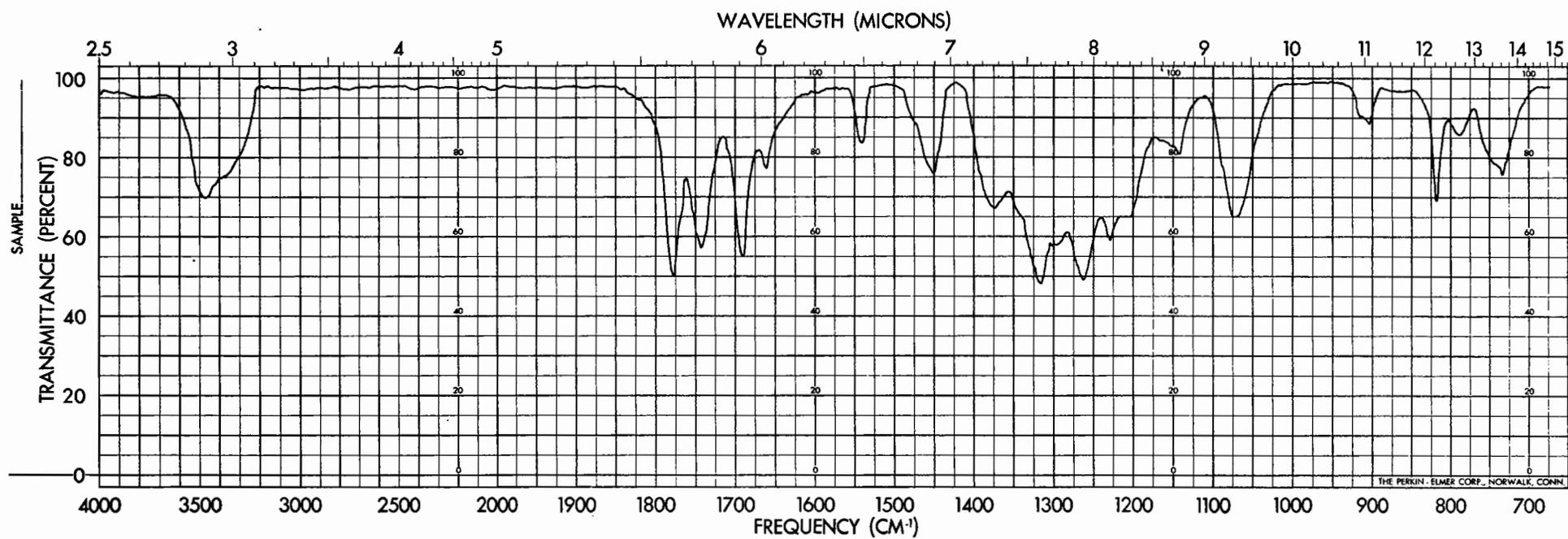
Figure 14. Infrared Absorption Spectrum of Diethyl 5-Carboxy-3-Hydroxy-2,4-Furandicarboxylate.
