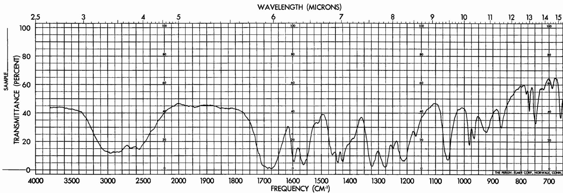
Figure 20. Infrared Absorption Spectrum of 3,4-Dimethoxy-2,5-Furandicarboxylic Acid.
