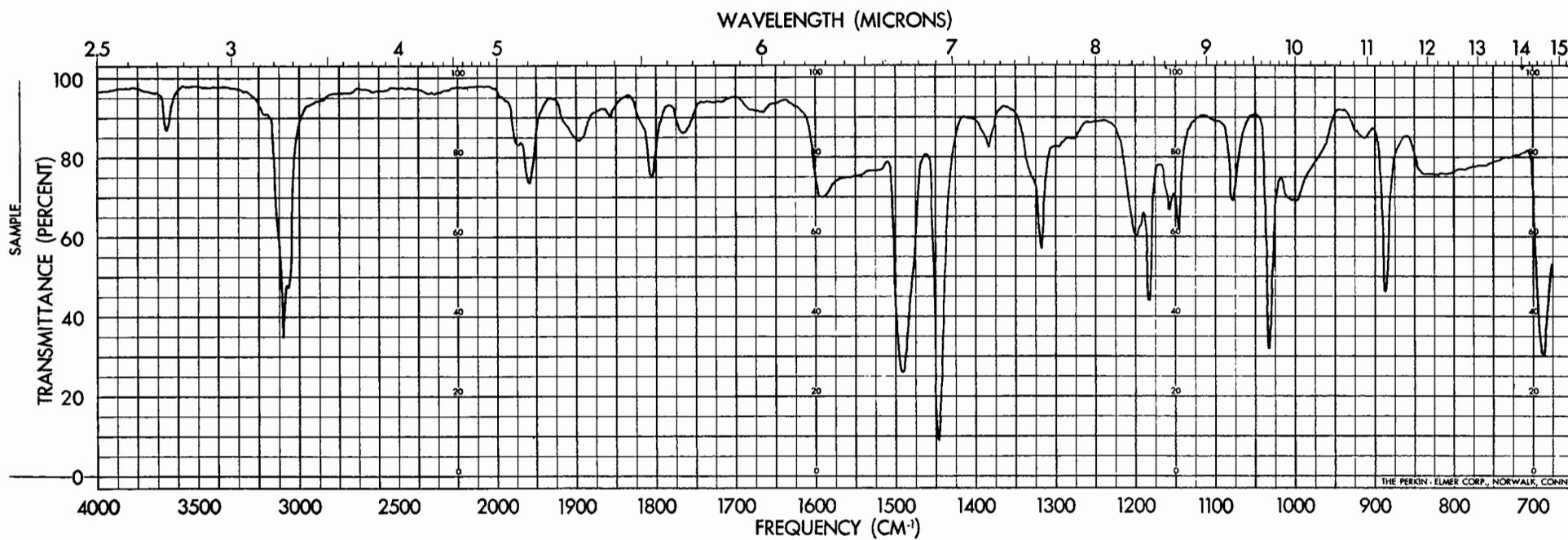
Figure 9. Infrared Absorption Spectrum of Product of Reaction between Triphenylmethyl Radicals and Dimethyl Peroxide.
