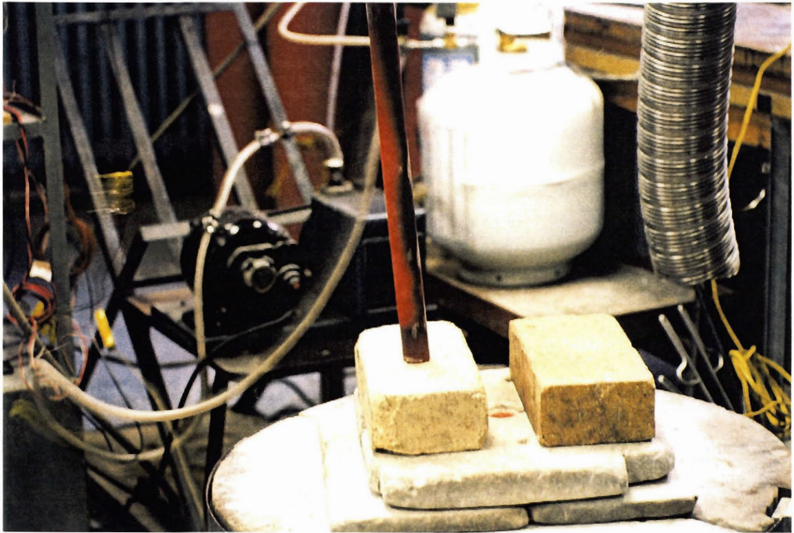
Figure 4.1 Hot-spot on the wall of a thermosyphon
