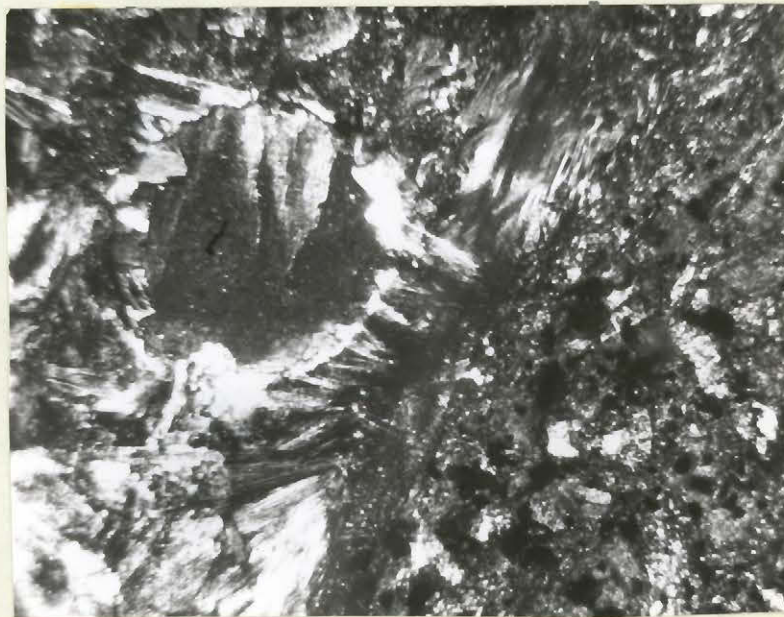
Plate XVlll: Duncan greenstone showing highly altered groundmass and altered amygdale.
