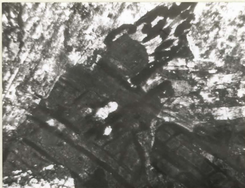
Plate XXXI1: Magnetite exsolved in pyroxene grains and producing a herringbone pattern. X45
