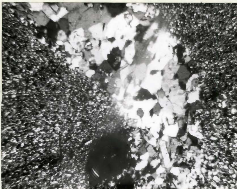
Plate Xll: Sandstone dyke filling fracture in siltstone. Characteristic of disconformities near bottom of Middle Mississagi. 16X
