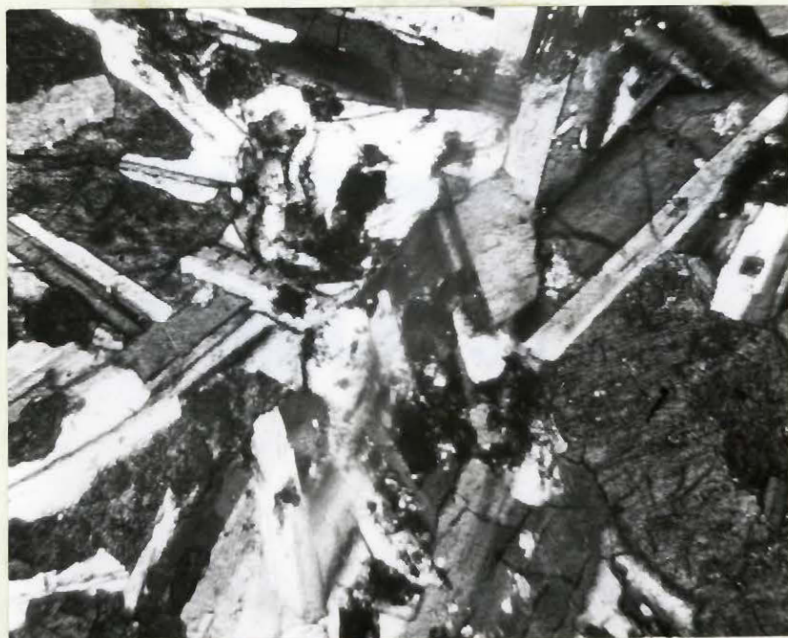
Plate XXXI: Photomicrograph of diabasic texture in amygdaloidal diabase dyke. Echo Lake area.
