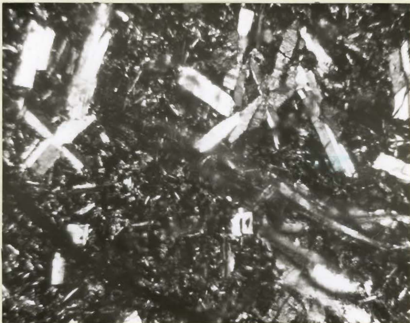
Plate XX: Slightly porphyritic Duncan greenstone showing laths of plagioclase in a groundmass of chlorite 64X.
