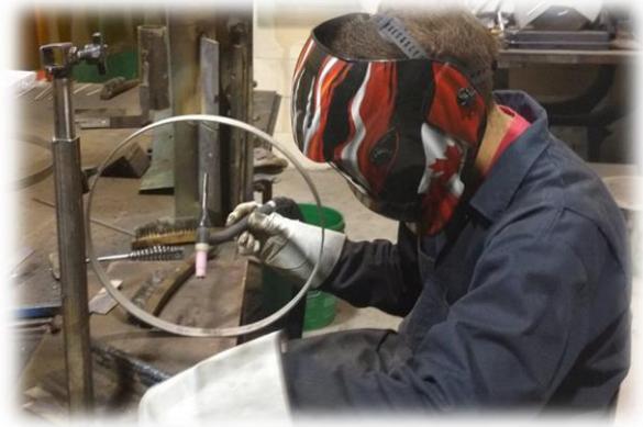
Figure 13a & 13b: TIG welding of supporting circles
