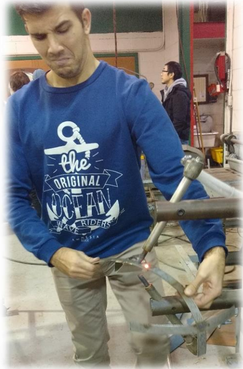
Figure 14a & 14b: Spot welding of vertical flat bars and brackets
