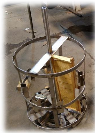
Figure 18: Finished basket holding a honey frame
