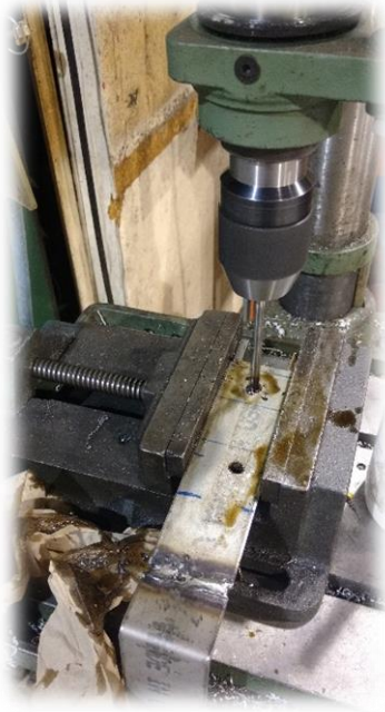
Figure 20: Drill press used to drill holes in the top bearing support flat bar
