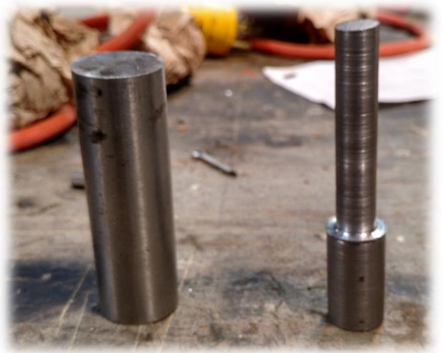
Figure 21a & 21b: Machining the drill connector piece using a lathe
