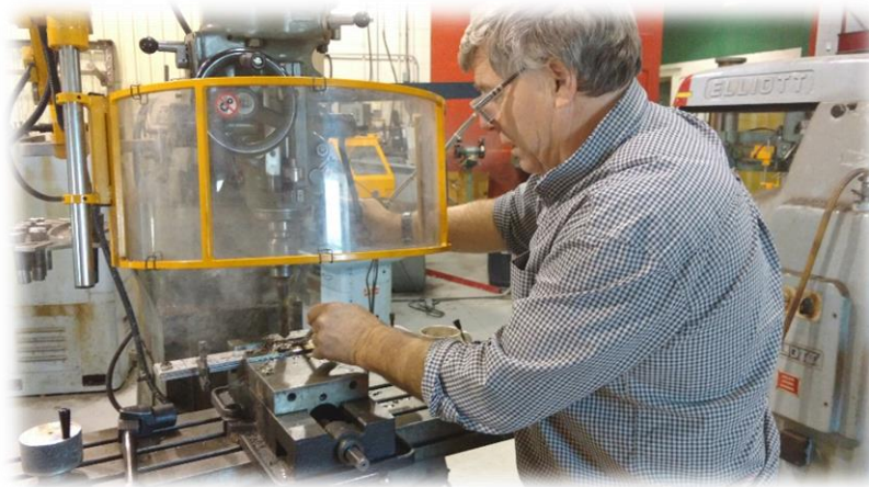
Figure 16: Drilling of the 1" hole in the stainless steel plates
