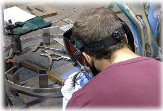
Figure 13a & 13b: TIG welding of supporting circles
