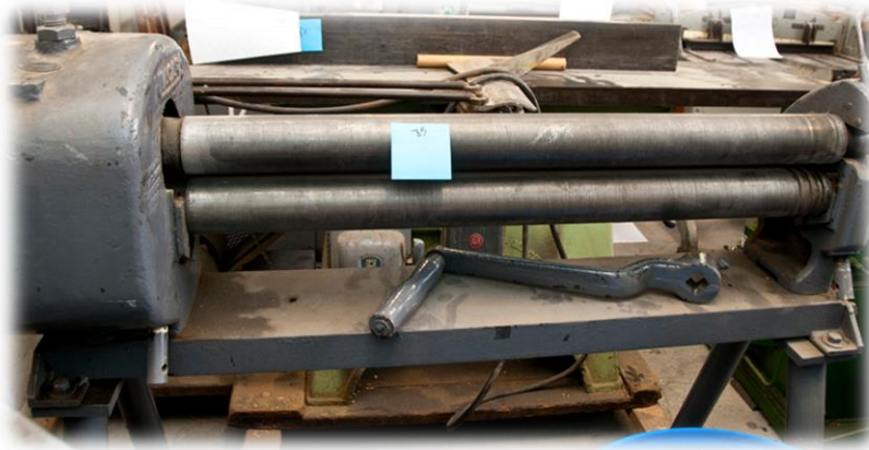
Figure 11: Roller used to make the three outer circles as well as the two bottom support circles
