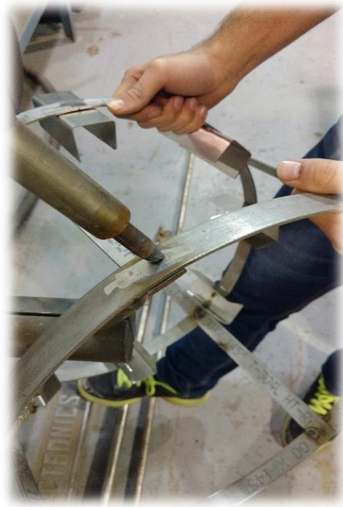
Figure 14a & 14b: Spot welding of vertical flat bars and brackets
