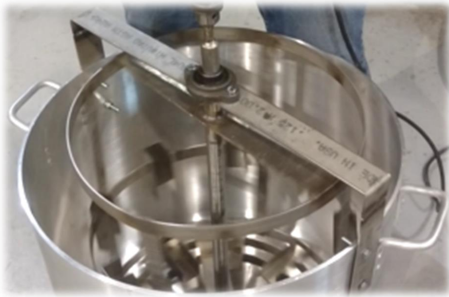
Figure 19: Top bearing mounted on support
