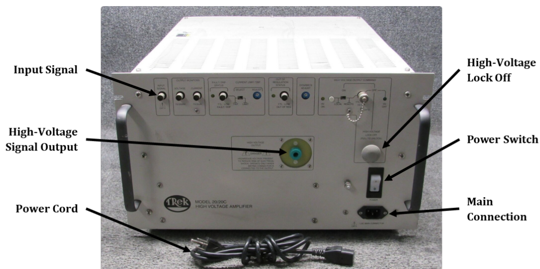
Figure. 3.18: Trek high-voltage amplifier labeled image showing the input port, high-voltage outlet, power cord, main connection, power switch, and high-voltage lock off. This device amplifies the AC signal generated by x2000. [69]
