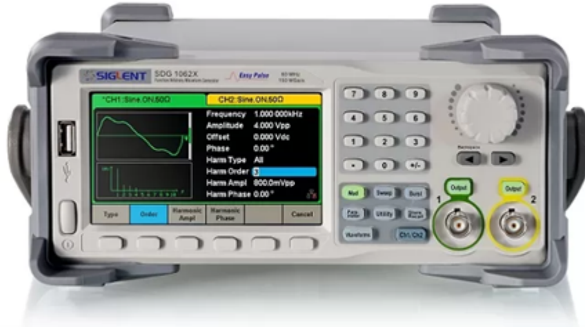
Figure. 3.17: SIGLENT signal generator. used to generate the AC signal to be amplified and used to drive the PGD reactor. The signal generator allows the amplitude and frequency of a sinusoidal signal to be set by a user. [67]
