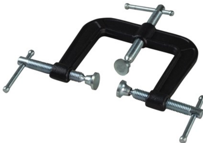
Figure. 3.15: Three-way C-clamp used to secure the gas injector to the rest of the reactor assembly. The two opposing heads on the clamp rest on the top and bottom quartz surface with pressure to secure the clamp. The remaining head pushed sideways on the gas injector to push it flush onto the reactor at the inlet. [66]
