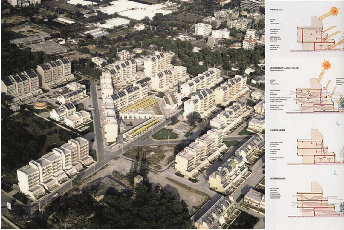
Figure 2.7: The Solar village in Athens, Greece. The urban solar grid enable a passive-solar design of the residential houses. (Source: Ruano, Miguel. Ecourbanism: sustainable human settlements, 60 case studies ).
