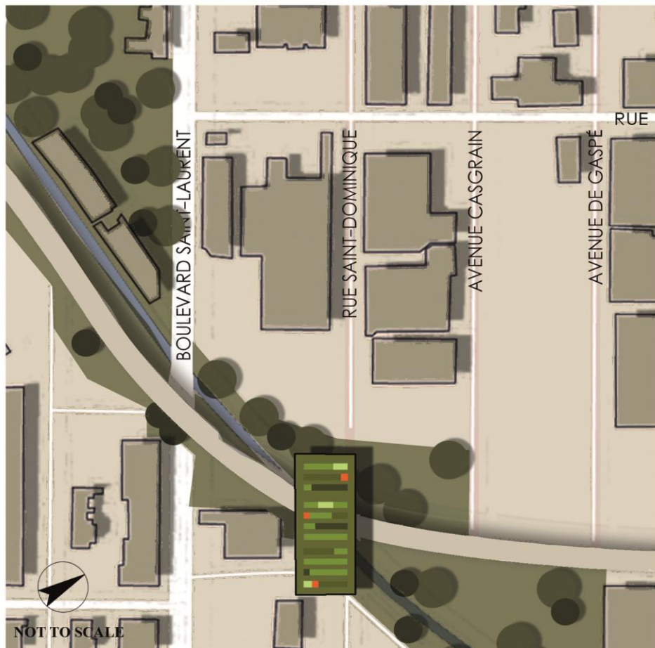
Figure 3.35: The proposed bridge will be partly covered for pedestrian crossing, and therefore protected from summer sun or winter rain. It will be accessible from both side of the railway by stairs and elevators.
