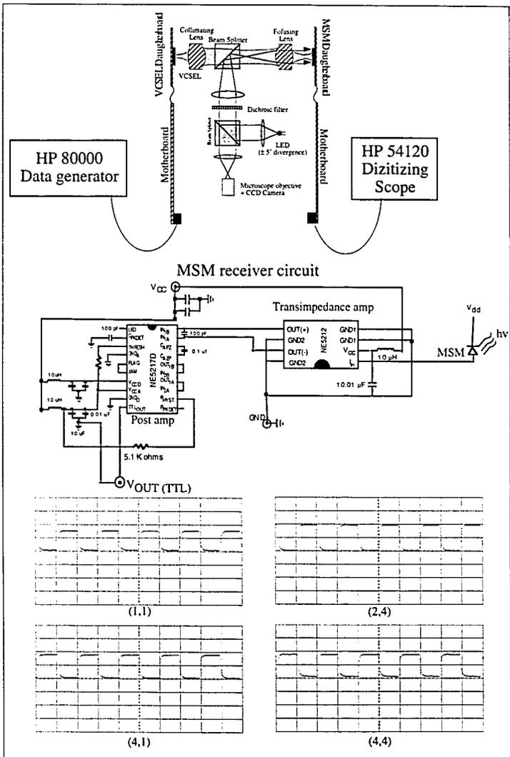
Figure 4.1.6 Measurement of 4 amplified receiver channels @ 155Mbit/sec.
