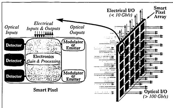
Figure 1.3.2 Smart pixel arrays integrated with the concept of M/D<sup>[16]</sup>.
