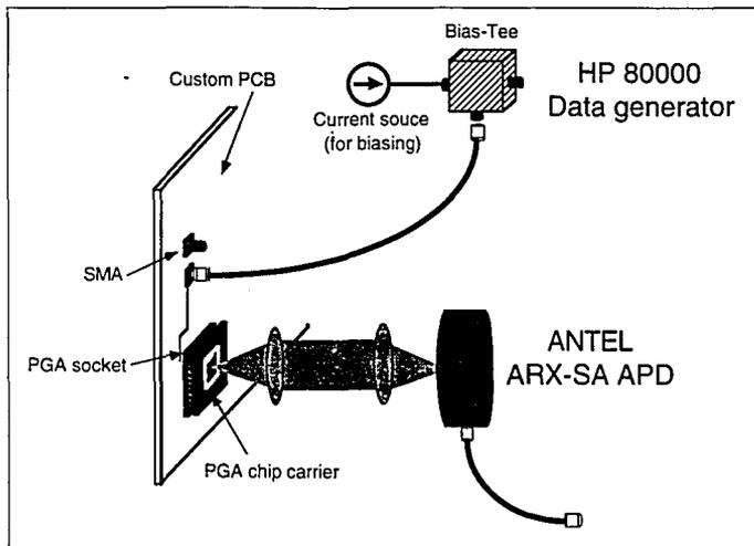
Figure 4.1.3 Prototype PCB used to test the speed of the VCSEL packaging.
