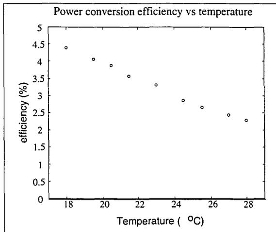
Figure 4.2.1 Power conversion efficiency vs. temperature.
