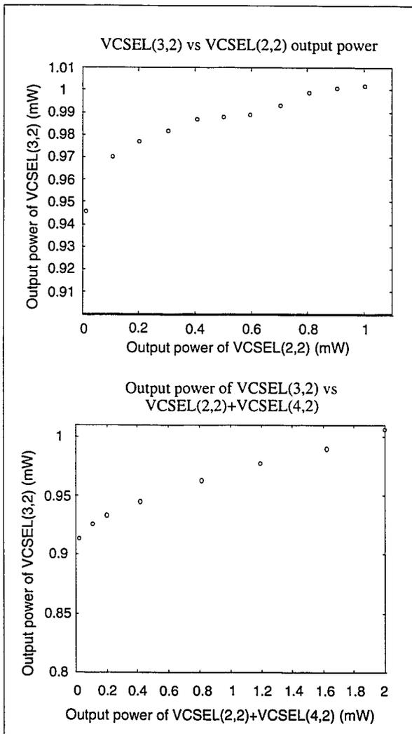
Figure 4.7.2 Optical power fluctuation due to operation of neighboring VCSELs.
