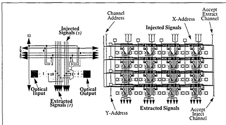
Figure 1.1.2 Schematics of a smart pixel array for implementing the Hyperplane architecture<sup>[16]</sup>
