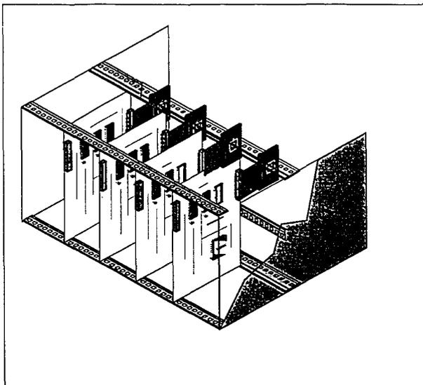
Figure 1.3.1 Conceptual view of the mother/daughterboards in a free-space optical backplane.
