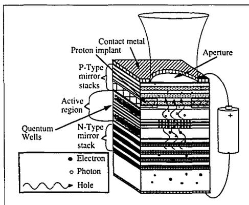
Figure 2.2.1 Cavity structure of a gain-guided VCSEL
