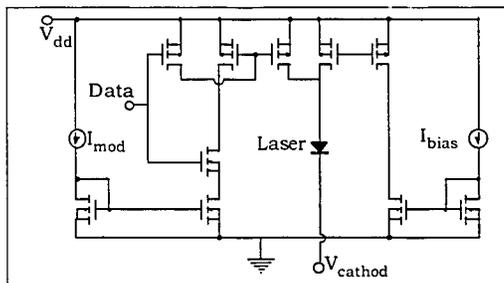
Figure 2.4.2 The current steering circuits used by the SPDA-16 driver from VIXEL corp.
