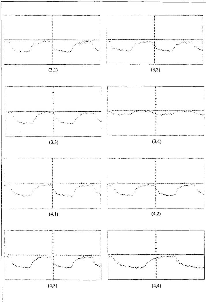
Figure 4.1.5 Output waveform of VCSELs individually modulated at 155Mbit/sec. with peak power of 800 $\mu$ W.
