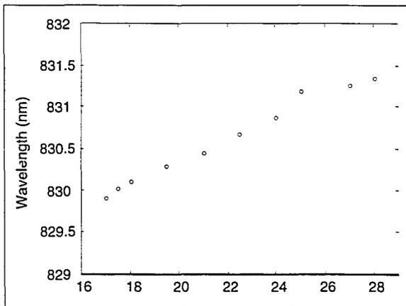
Figure 4.3.1 Die temperature vs. output wavelength.
