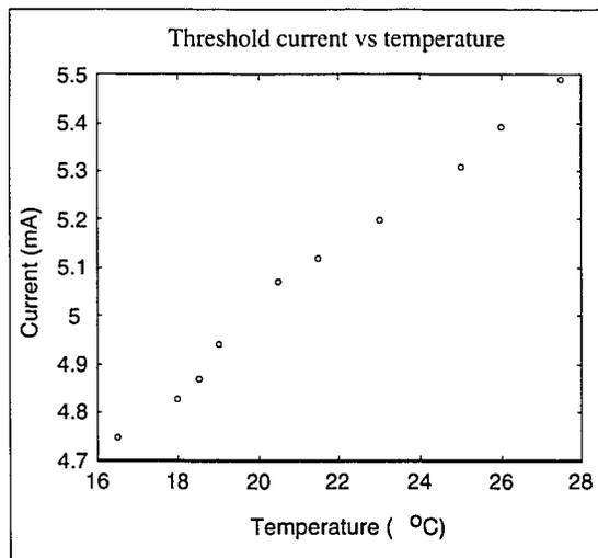
Figure 4.6.1 Threshold current at different temperature.
