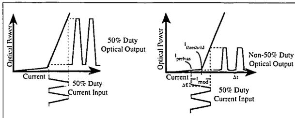
Figure 2.4.1 Input current bias levels and the optical output of diode lasers
