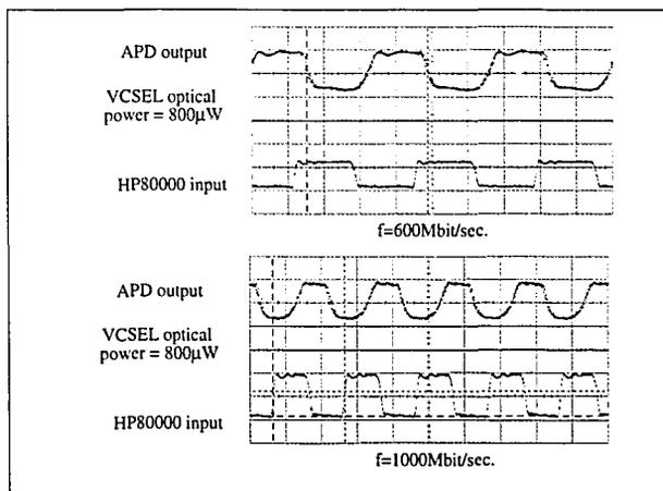
Figure 4.1.4 Modulation waveform of the setup in Figure 4.1.3 (power on the detector is 700uW).
