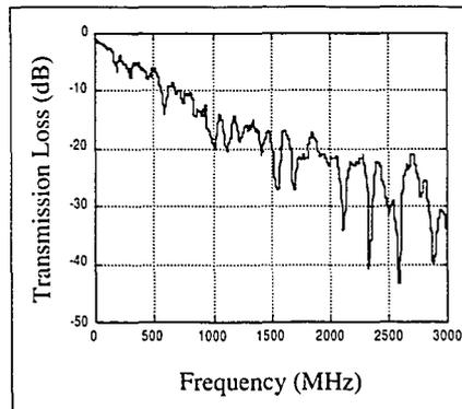
Figure 3.1.6 Frequency measurement of the mother/daughterboard assembly.
