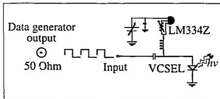
Figure 3.1.4 Circuit diagram of a single transmitter channel
