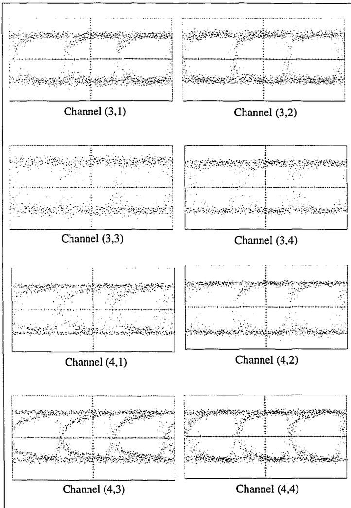
Figure 4.1.7 Eye pattern generated with  $2^{23}-1$  pseudo-random bit stream at a 155Mbit/sec .
