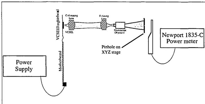
Figure 4.7.1 Measurement setup used to measure crosstalk between VCSELs.
