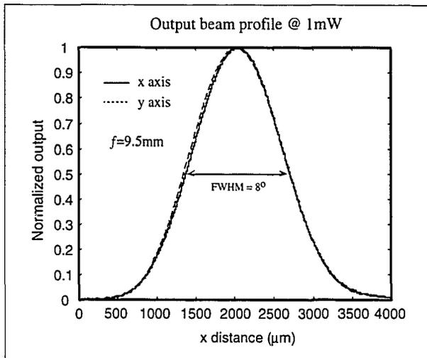
Figure 4.4.1 Output beam profile of the VCSEL at 1mW output power.
