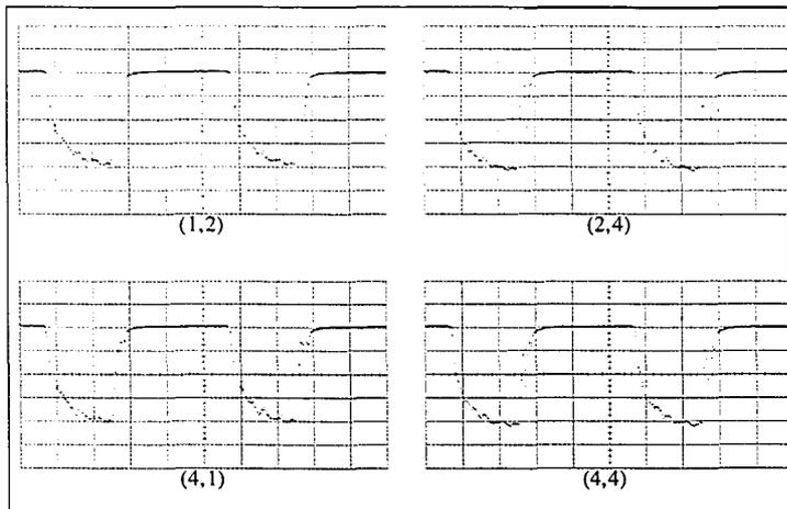
Figure 4.15 Simultaneous operation of 4 channels at 1Mbit/sec with 480uW of optical power.
