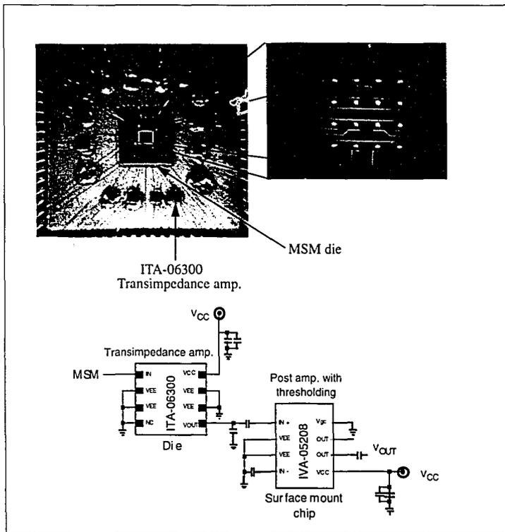
Figure 4.1.6 Packaging and schematic diagram of the receiver board.
