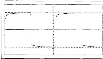
Figure 4.14 Output waveform of a 50 Ohm terminated SPDA-16 output at 7Mbit/sec.
