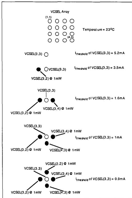
Figure 4.6.2 Threshold currents at operation of different neighboring VCSELs.
