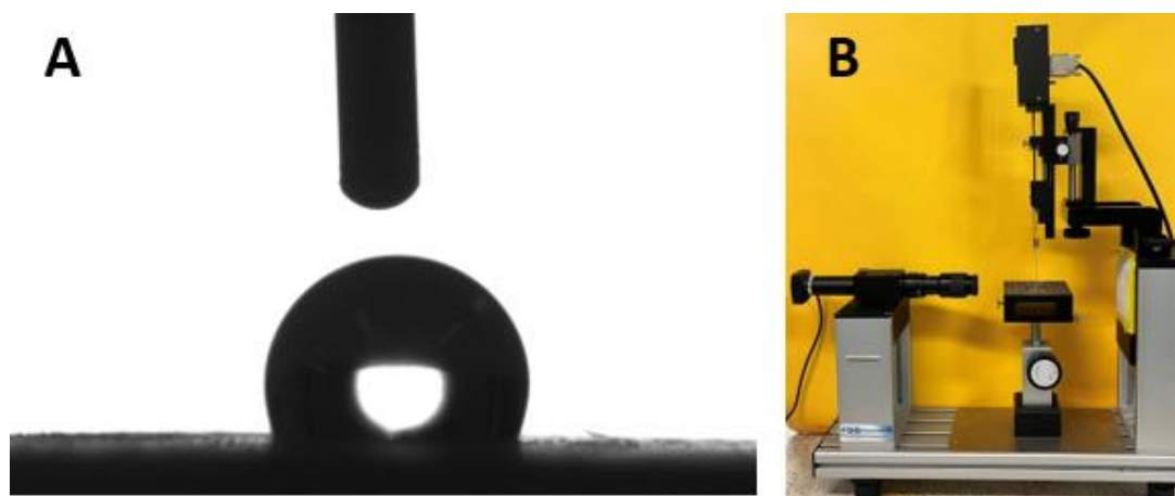
Figure 6-3. a. Representative photograph of the water droplet spread; b. Goniometer.
