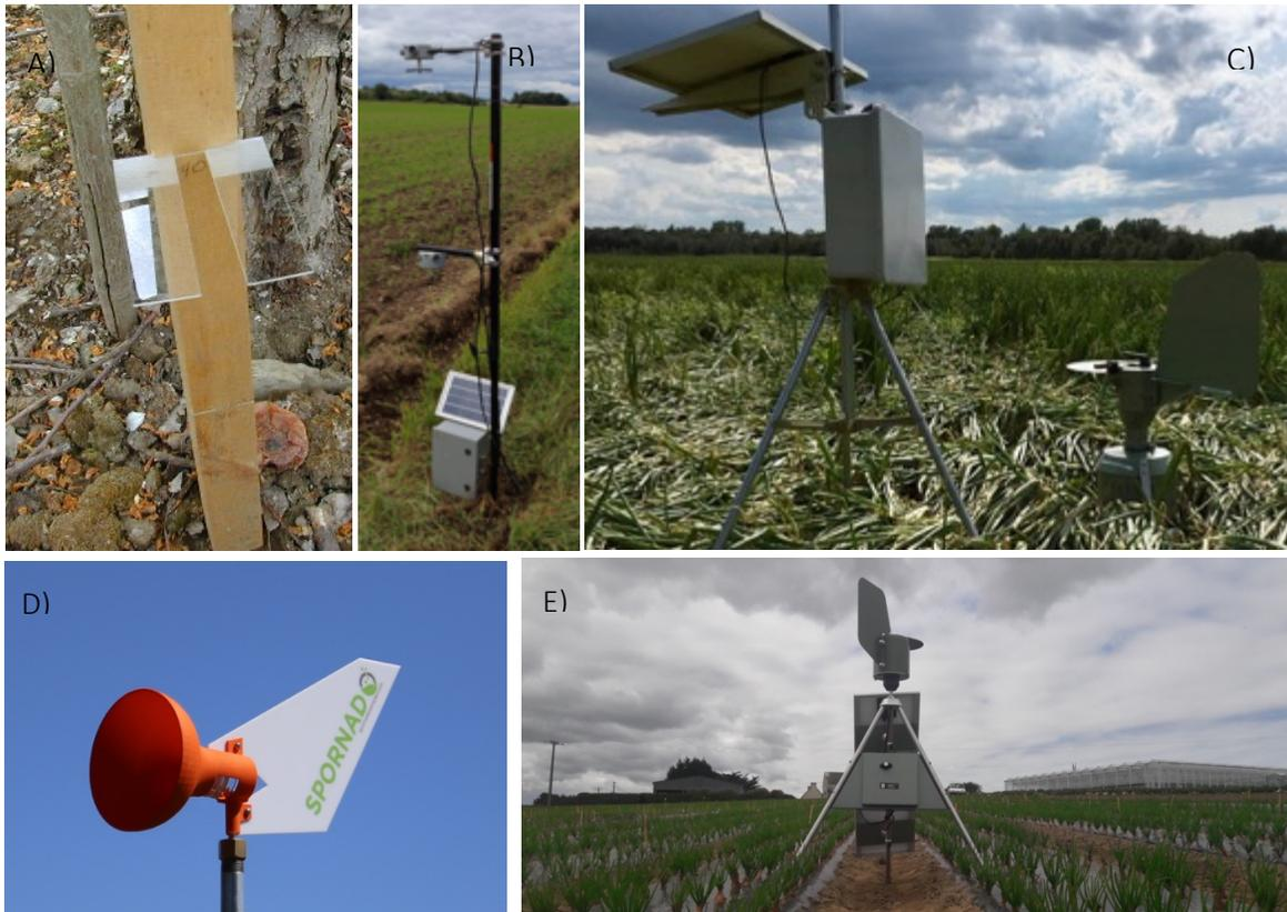
**Figure 3-1.** Examples of spore samplers. A) Passive sampler comprising two microscope slides mounted horizontally on a wooden pole; B) rotating-arm impactors; C) Burkard 7-day recording volumetric sampler; D) funnel-like passive spore sampler from Spornado (courtesy of Kristine White and Yaima Arocha Rosete, Sporometrics); and E) Burkard high-volume cyclone (courtesy of Celine Hamon, Vegenov).
