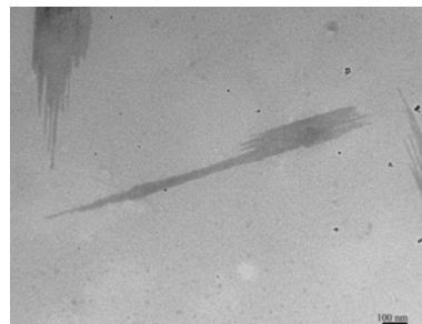
(b) TEM image of ENCC. (c) ENCC at Cu(II) = 100 ppm. (d) ENCC at Cu(II) = 300 ppm.
