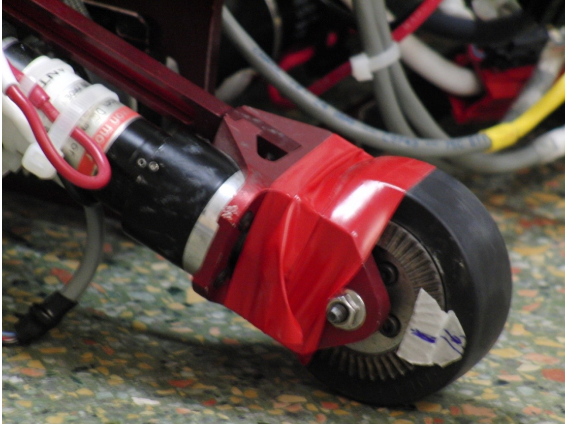
FIGURE 4.5 MECHANICALLY BLOCKED WHEEL
