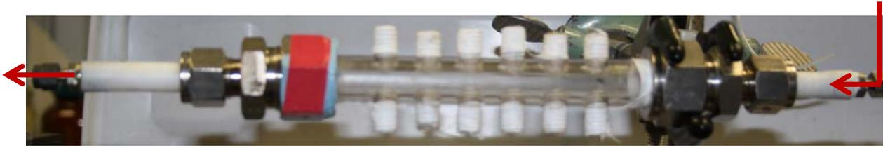
Figure 4.6. The picture of the peculiar column with six sample ports in the both top and bottom sides.
