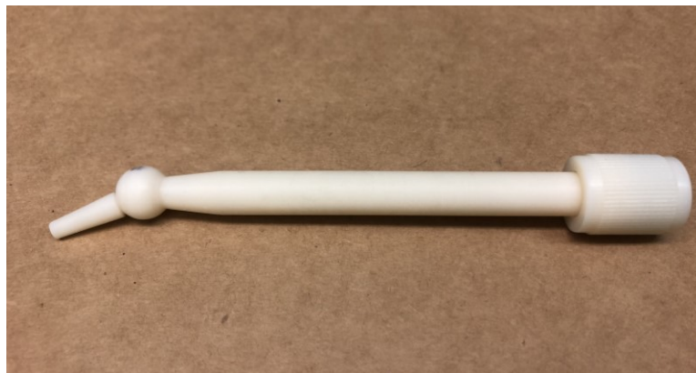
Figure 54: Re-designed NFLJI nozzle prototype prepared by Medical International Technologies (MIT Canada) Inc. This nozzle targets an injection angle of 15 degrees relative to the lower occlusal plane of the central incisors.
