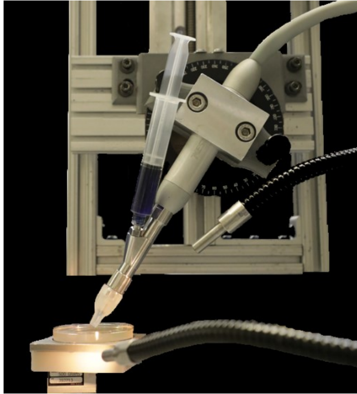
Figure 10: Experimental test bench configuration for assessing the impact of nozzle angulation from 0 to 75 degrees on outcomes of the NFLJI system (Meso-Jet, MIT Canada Inc, Canada).
