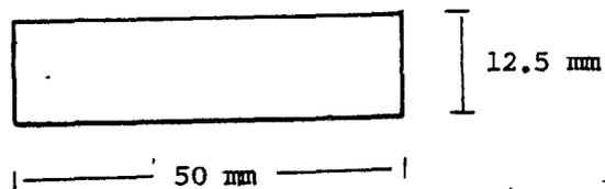
Figure (5.12b). Actual Dimensions of 1.6 mm (1/16 in.) Thick Flexural Test-pieces.
