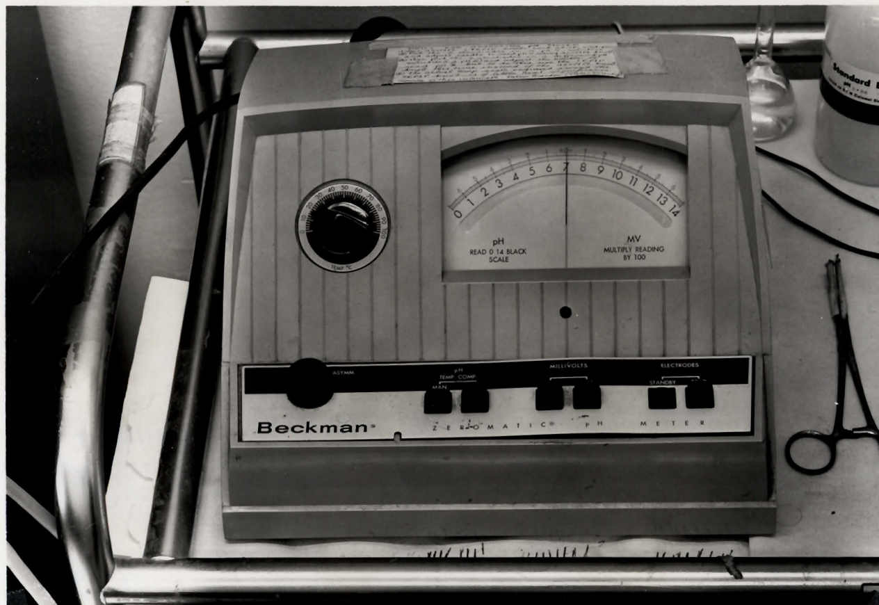
Fig. 3: The Beckman Zeromatic pH meter used for pH determinations. The unit is accurate to 0.1 pH units and has a reproducibility of 0.02 pH units. It was coupled to a Sanborn multichannel recorder for simultaneous recording of pH and esophageal pressures.
