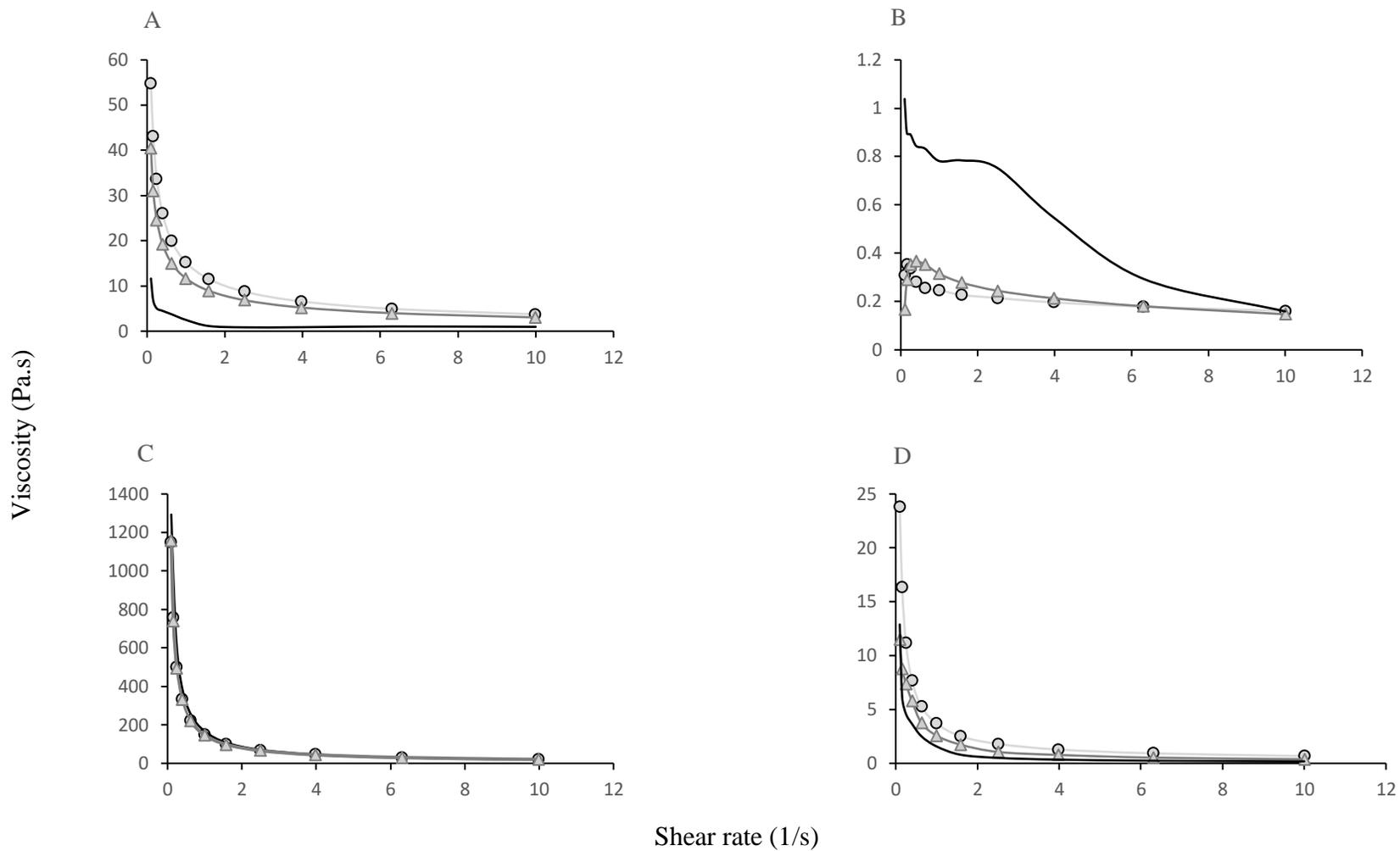
**Fig. 4:** Effect of shear rate on viscosity at different levan concentrations and temperatures; (A) 10% HMW levan; (B) 5% HMW levan; (C) 10% Mix L/HMW levan and (D) 5% Mix L/HMW levan at  $\circ$  25°C,  $\triangle$  50°C and  $—$  75°C.
