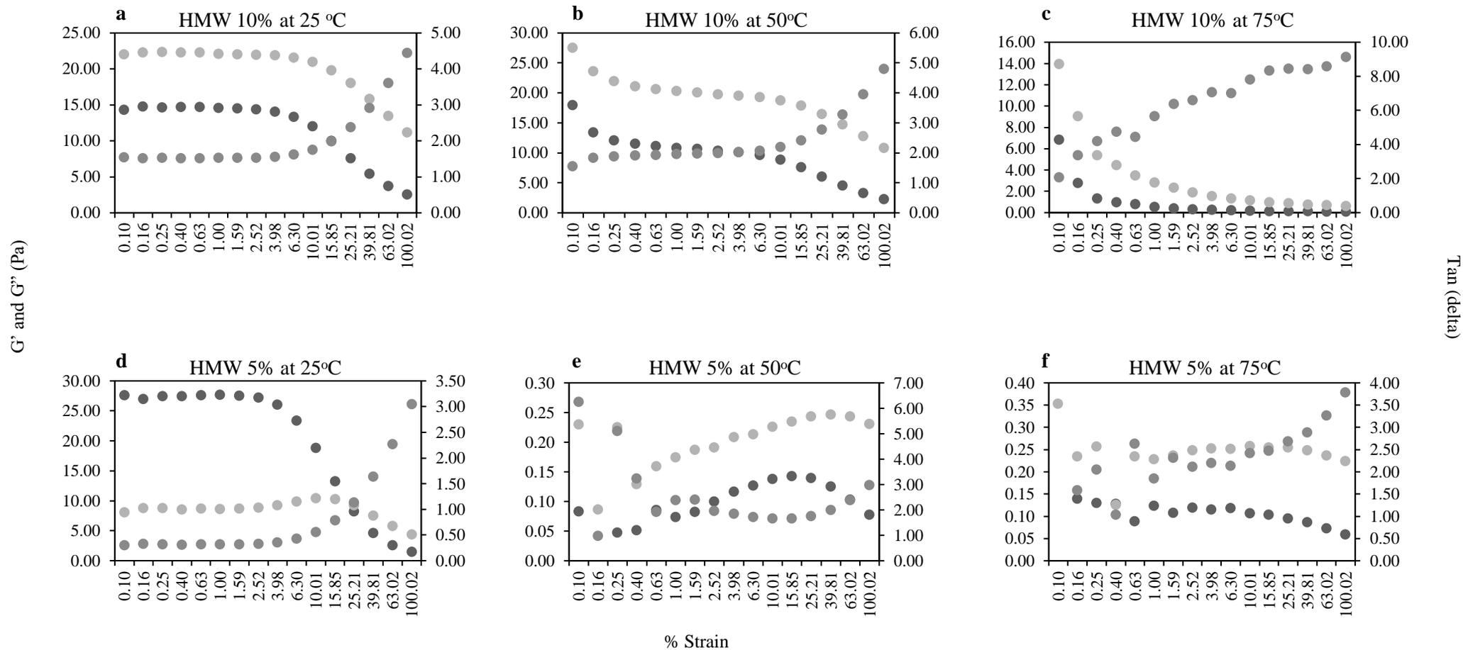
**Fig. 5:** Strain sweep measurements at 1.0 Hz of HMW levan at different concentrations (10 and 5% w/v) and different temperatures (25, 50 and 75°C) ● average  $G'$ ; ● average  $G''$ ; ● average tan ( $\delta$ )
