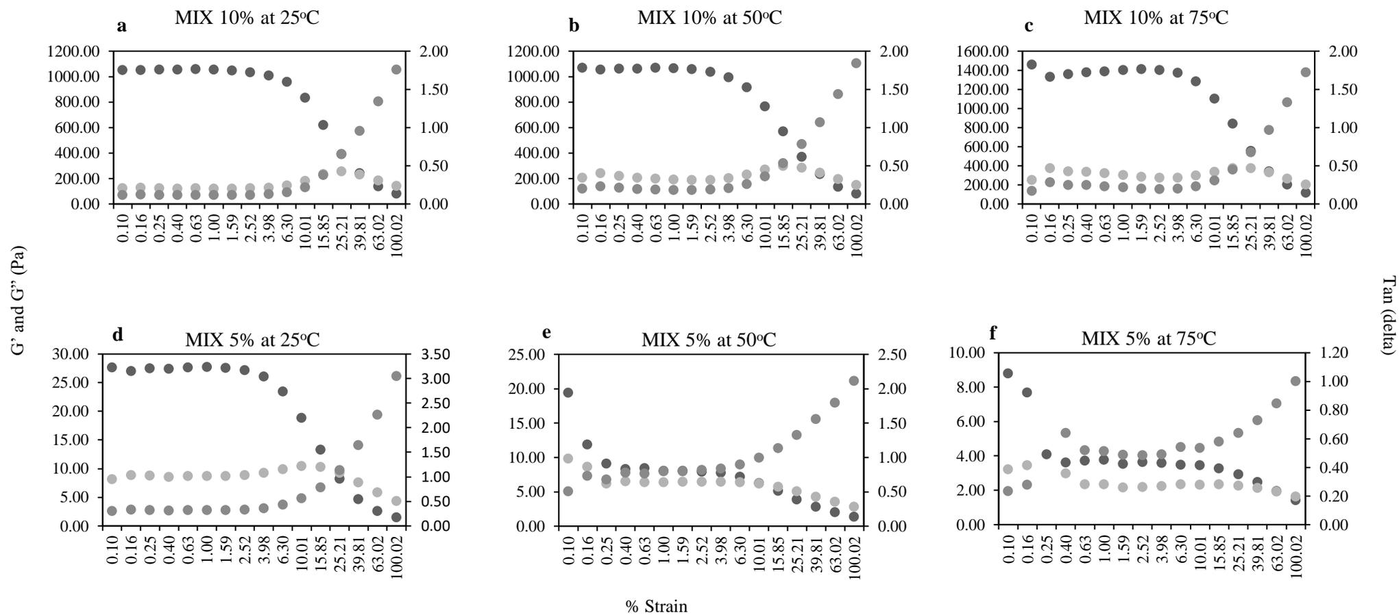
**Fig. 6:** Strain sweep measurements at 1.0 Hz of mix L/HMW levan at different concentrations (10 and 5% w/v) and different temperatures (25, 50 and 75°C) ● average  $G'$ ; ● average  $G''$ ; ● average  $\tan(\delta)$
