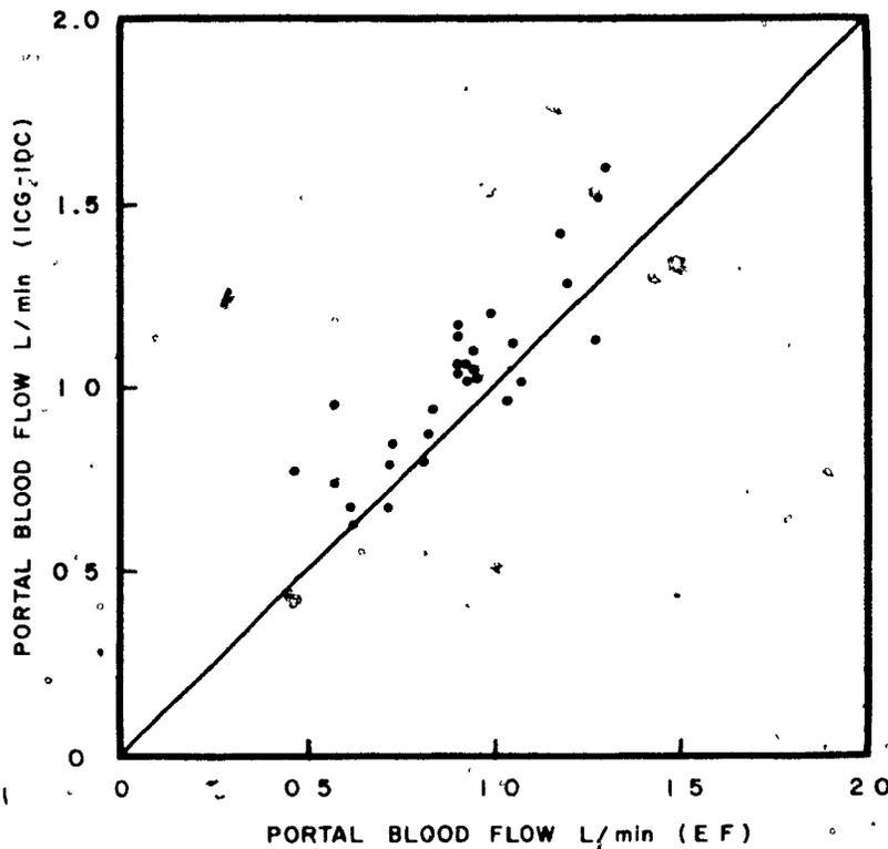
FIGURE 20: COMPARISON OF PORTAL BLOOD FLOWS OBTAINED SIMULTANEOUSLY BY ELECTROMAGNETIC FLOWMETERS (E.F.) AND INDOCYANINE GREEN INDICATOR DILUTION CURVES (I.C.G.-I.D.C.) (GROUP G). THE SOLID LINE IS THE LINE OF IDENTITY.
