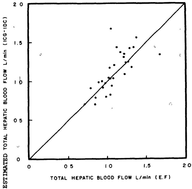
FIGURE 18: COMPARISON OF TOTAL HEPATIC BLOOD FLOWS OBTAINED SIMULTANEOUSLY BY ELECTROMAGNETIC FLOWMETERS (E.F.) AND INDOCYANINE GREEN INDICATOR DILUTION CURVES (I.C.G.-I.D.C.) (GROUP G). THE SOLID LINE IS THE LINE OF IDENTITY.
